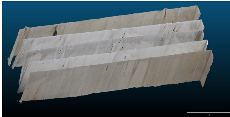
Figure 4. 3D photogrammetric model of extractive fronts.
