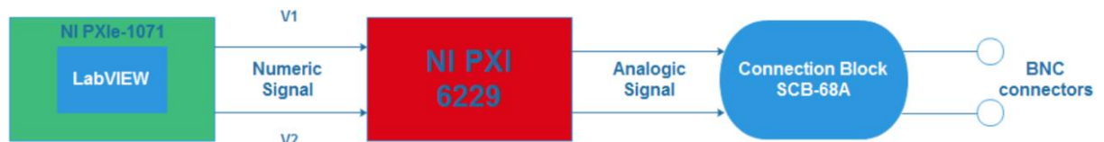
Figure 2.10 Scheme of the data flowing process between LabVIEW and the table's controller.
