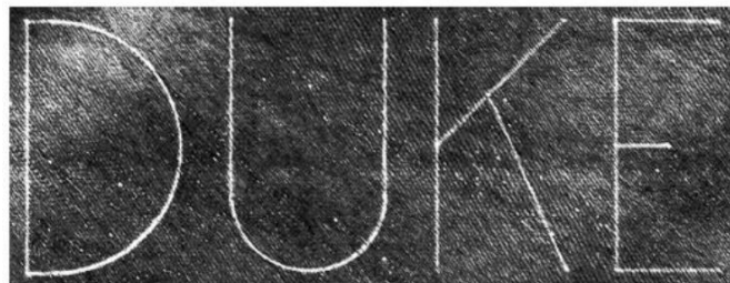
Figure 1.4 AFM image of the obtained pattern [extracted from (Johannes M. S., Kuniholm, Cole, & Clark, 2006)].
