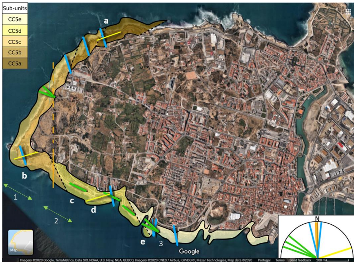
Figure II.2.3. Satellite map of the Peniche peninsula (Google, 2020) with indication of sub-units cropping out along the peninsula margin. The cliffs along green arrows 1 and 2 are shown in Figure II.2.5. Images of location 3 in the southern margin, corresponding to the base of the CC5e sub-unit, are shown in Figure II.2.6. Faults and fractures strike directions were registered along the Peniche peninsula margins, with fractures at locations ‘a’ to ‘e’ represented in Figure II.2.7. A major fault zone is marked by the orange line, two fracture sets are marked by green and blue lines; calcite-filled fracture sets are marked in yellow. The strike directions of these fracture sets are represented on the bottom-right diagram.
