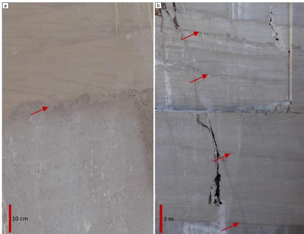
Figure IV.1.10. Examples of discontinuities observed on outcrop at Codaçal (red arrows), with indications of erosion/reworking in some.
