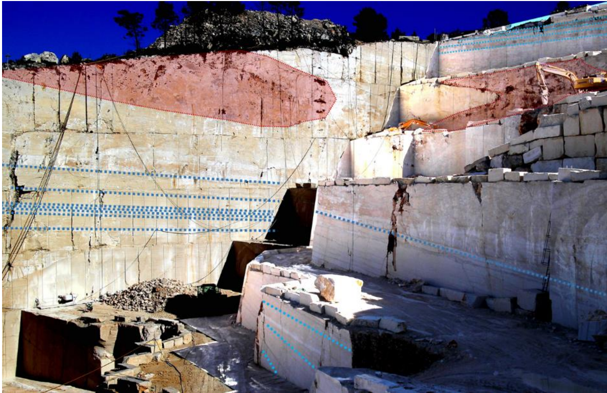
Figure IV.1.9. Vertical succession and overall geometries of the Codaçal Member. Generally tabular geometries in the lower half (bedding planes represented by blue lines) and biostromes and coral/algal build-ups towards the top (red polygons). Vertical height of the quarry front is an estimated 35 to 40 m.
