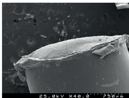
Figure 3.13. Scanning electron microscope image of cohesive fracture (original magnification x40)
