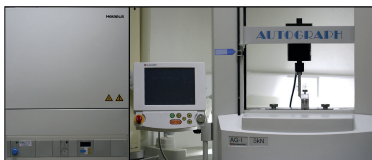
Figure 2.2. a) Thermo Scientific Heraeus® BK 6160. b) Universal test machine (Model AG-I, Shimadzu Corporation, Kyoto, Japan).
