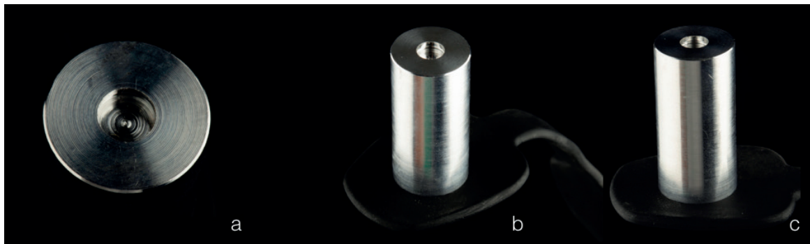
Figure 2.1. a) A detail of 360° groove at the bottom of the central cavity; b) and c) Aluminum blocks specifically fabricated within the scope of this kind of studies (photographs courtesy of Professor Paulo J. Palma).
