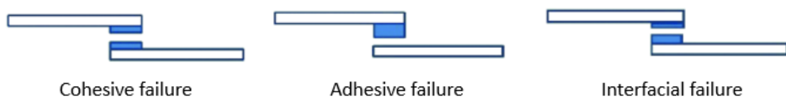
Figure 2.3. Adhesive bonding failure modes: a) Cohesive failure; b) adhesive failure; c) interfacial failure (adapted from [27]).
