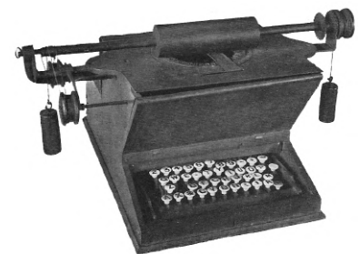
Figure 22: Improved version of typewriter from 1870s with QWERTY keyboard layout [Commons, 1868b]
