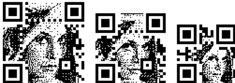
Figure 28. Results of the Halftone QR Code for the same image using different levels.
