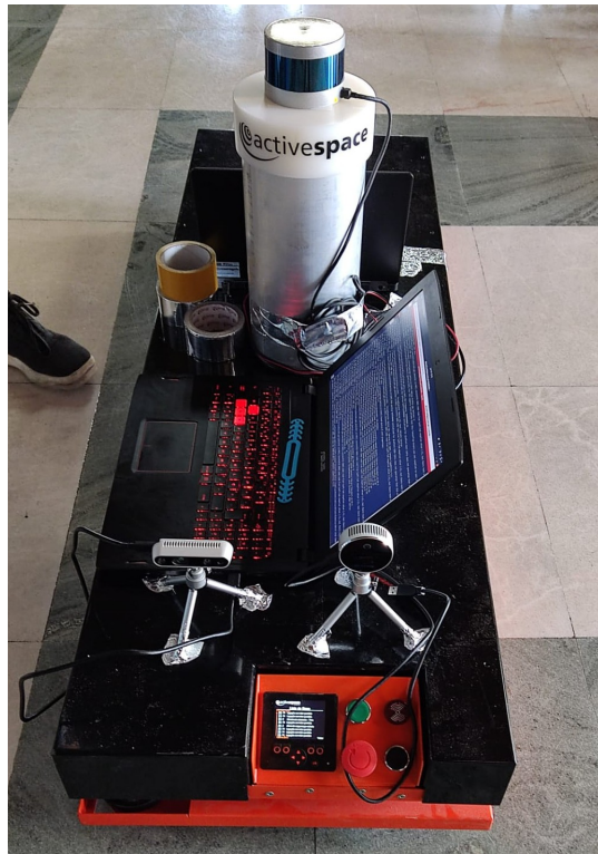
Figure 3.9: AGV with a VLP-16, L515 and a D435i.
