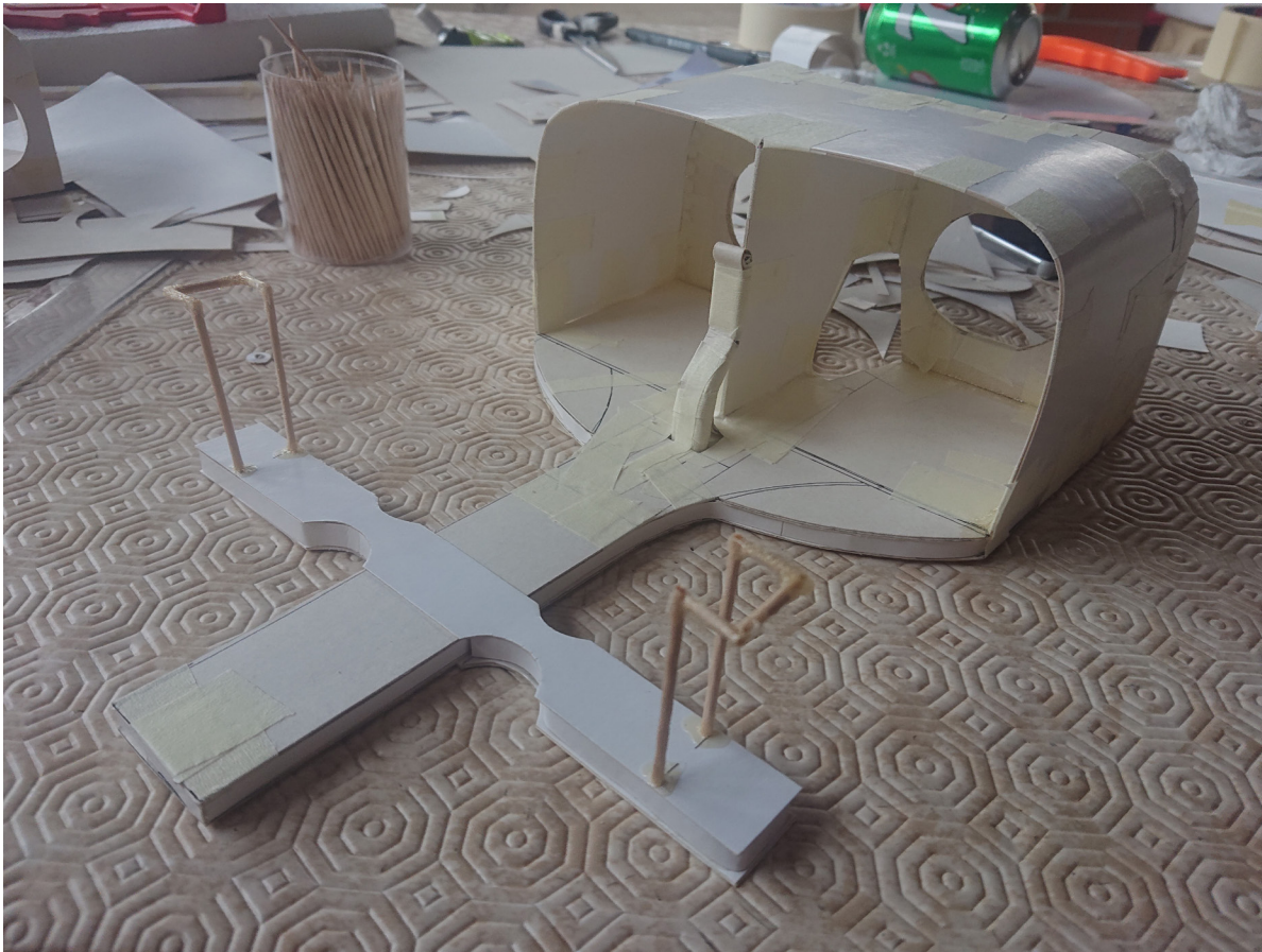
Fig. 61 Finished model of first design with stronger structure and enhanced smartphone support mechanism
