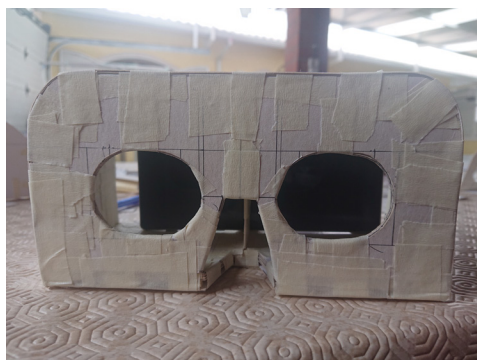
Fig. 76 & 77 New head prototype with bigger dimensions that was capable of holding all the existing smartphones
