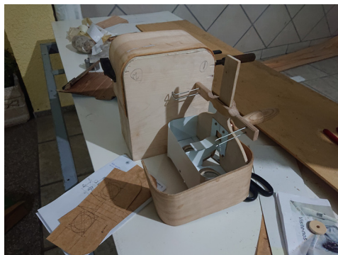
Fig. 131 (left) Wood top piece drying in one of the mould pieces
