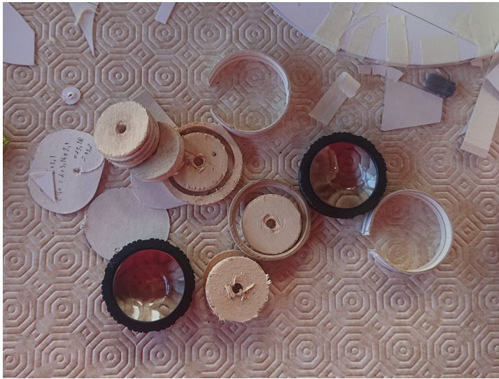
Fig. 86 Lenses taken from VR headsets and the paper cases we built for them, as well as wood casing prototypes
