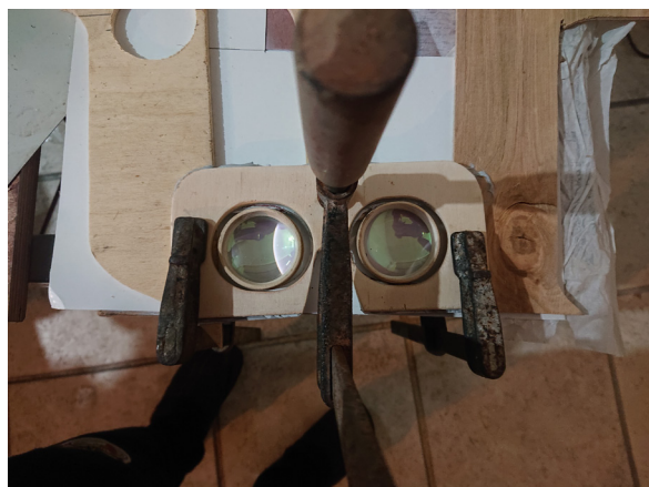
Fig. 97 (right) Glued metal sheet in the face piece with lenses already inserted
