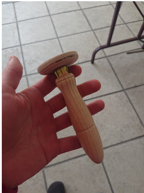
Fig. 100 (left) Prototype wood handle. The top piece was made by us and the bottom one was bought
