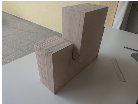
Fig. 129 (left) Wood mould built for the device top piece
