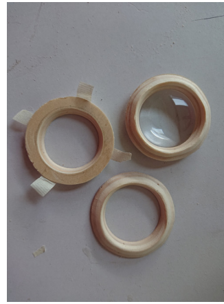
Fig. 123 (left) Wood cuts for new lens casing
