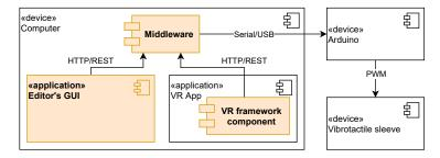
Fig. 1: Architecture of the Vibrotactile Editor System
