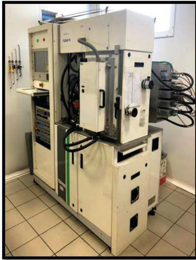
Figure 3-1: TSD-400 small size industrial deposition machine with one target and additional plasma source.
