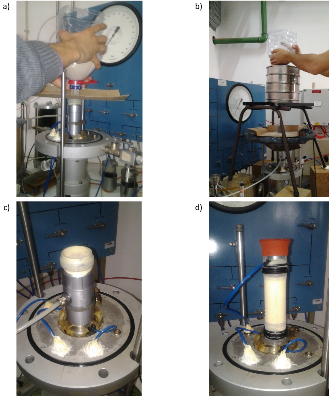
Figure 2.5 – Sample set-up: (a) air-pluviation of loose sand using a miniature container; (b) air-pluviation of dense sand by applying the multiple sieve technique; (c) detachable mould supporting the sample; and (d) application of vacuum after disassembly the mould.
