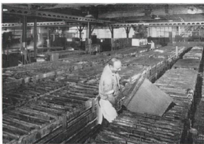
Fig. 2.1. Electroplating cells, where several plates were used as cathodes and anodes [4].
