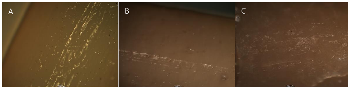
Figure 3.11. PLM images of solid dispersions manufactured by HME: A, SLP + 50% IBR + 10% PEG6000; B, PVPVA + 50% IBR + 15% P40; and C, PVP + 50% IBR + 10% PEG6000. The scale bars of PLM represent 100 \mu\text{m} .
