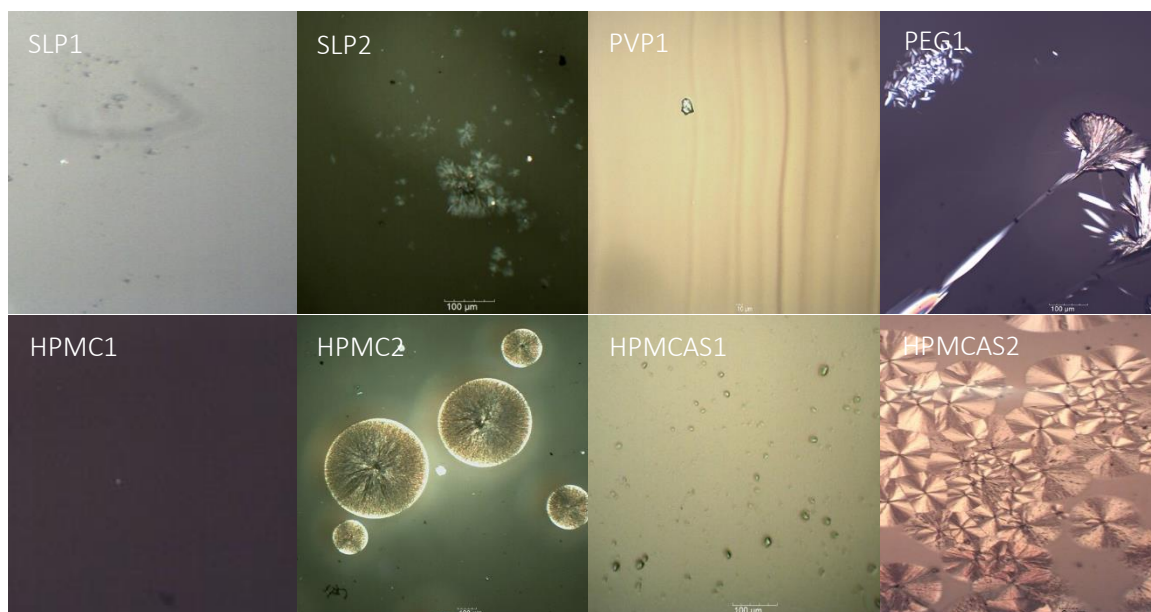
Figure 2.9. Birefringence of some binary compositions detected by polarized light microscopy. SLP1: Sample SLP + 1% ETR at T0 with no crystals detected, objective 50x; SLP2: Sample SLP + 50% ETR after 7 days of storage in the 25°C/ 60% RH climatic chamber, objective 10x; PVP1: Sample PVP + 25% ETR after 4 days of storage at room temperature with no crystals detected, objective 10x; PEG1: Sample PEG + 50% ETR at T0, objective 5x; HPMC1: Sample HPMC + 30% ETR at T0 with no crystals detected, objective 10x; HPMC2: Sample HPMC + 50% ETR after 7 days of storage in the 25°C/ 60% RH climatic chamber, objective 5x; HPMCAS1: Sample HPMCAS + 20% ETR after 4 days of storage in the 25°C/ 60% RH climatic chamber with no crystals detected, objective 10x; HPMCAS2: Sample HPMCAS + 50% ETR at T0, objective 10x.
