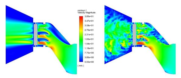
Figure 12 - Flow velocity for (left) steady-state RANS and (right) flow time 0.25s with DES model.
