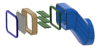
Figure 1 - Geometry of the airvent.
