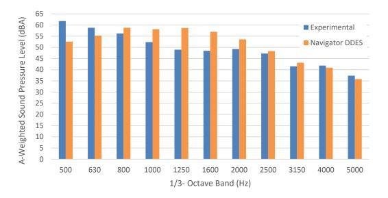
Figure 11 - Comparison between numerical and experimental data.
