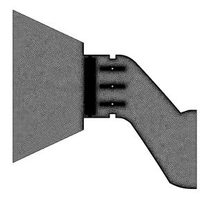
Figure 3 - Airvent interior discretized by 1.7 million cells.
