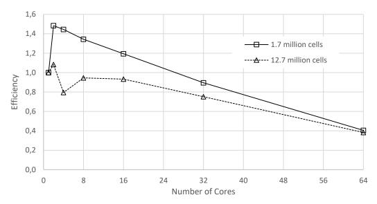
Figure 8 - Efficiency for two mesh densities, considering a single node.
