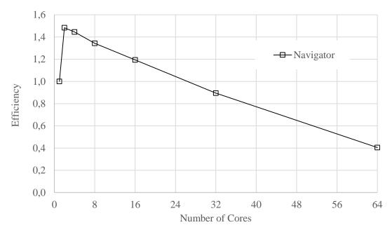
Figure 6 - Efficiency for a 1.7 million cell mesh, considering a single node.
