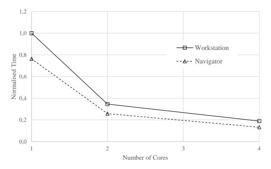
Figure 4 - Normalized execution time for the workstation and Navigator Cluster.
