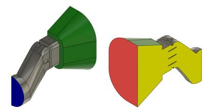
Figure 2 - Interior of the airvent with inlet (blue), outlet (red) and symmetry (yellow) conditions.
