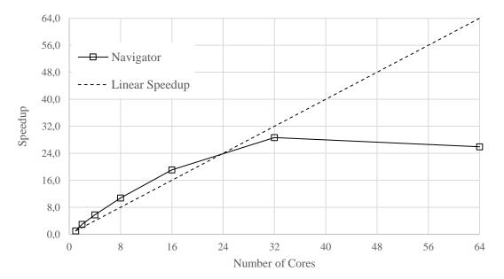
Figure 5 - Speedup for a 1.7 million cell mesh considering a single node.
