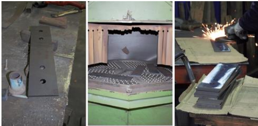
Fig. 2.2 – Preliminary treatment: a) plates before treatment; b) mechanical blasting; c) grinding.
