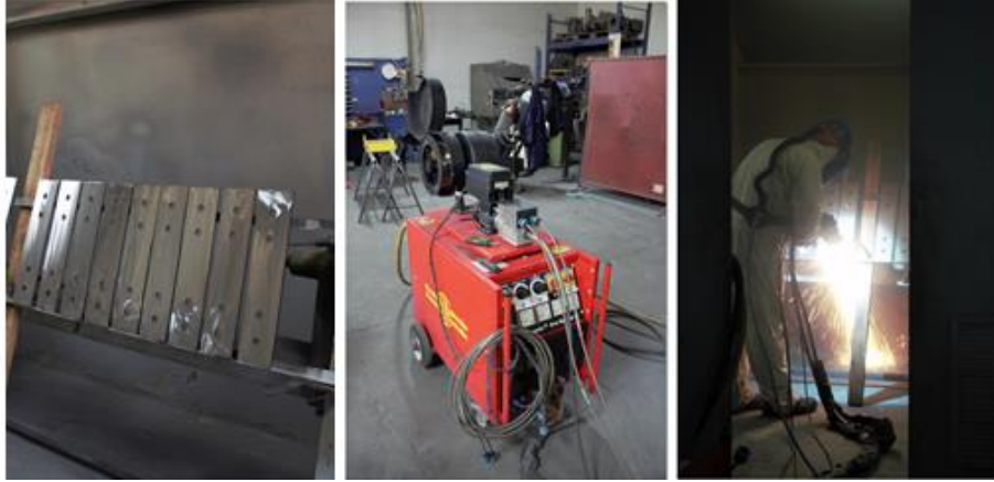
Fig. 2.3 – Electric arc wire spray: a) plates before spray; b) machine for electric arc wire spray; c) spray coating.
