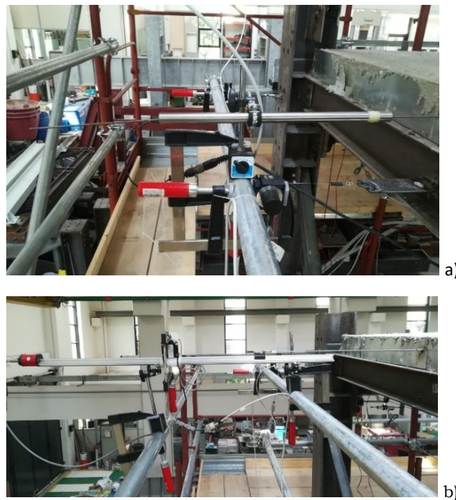
Fig. 5.177 – a) LVDT and wire transducers; b) MTS Temposonic transducer
