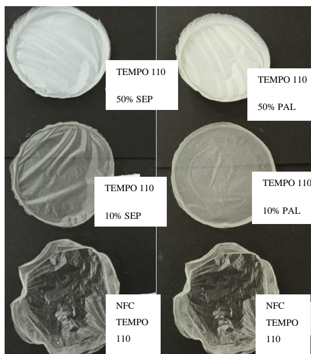
Figure 15d. Composite films for NFC TEMPO 110 with 0% mineral (bottom), 10% mineral (middle) and 50% mineral (top), produced through solvent casting.
