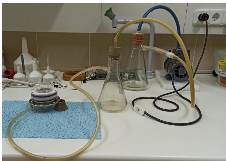
Figure 9. Filtration setup, consisting of two Kitasato flasks, a vacuum pump and a filter plaque with a porosity of 45 \mu m.
