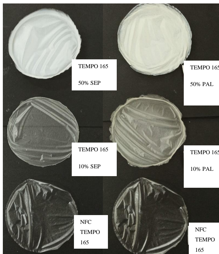
Figure 15e. Composite films for NFC TEMPO 165 with 0% mineral (bottom), 10% mineral (middle) and 50% mineral (top), produced through solvent casting.
