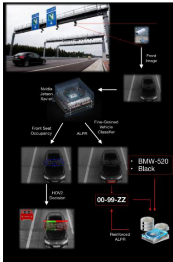
Figure 1: Example of parallel recognition systems for fraud detection. License plate and vehicle info are extracted and cross-examined.
