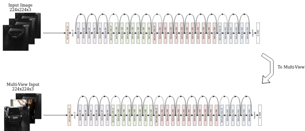
Figure 25: MC-CNN. Top Network is typical CNN usage with RGB image. Bottom is the suggested multi-view over multi-channels.
