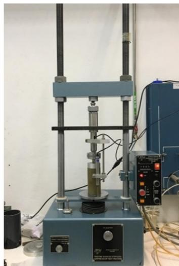
Figura 4.5 – Prensa Tristar 5000kg Stepless Compression Test Machine
