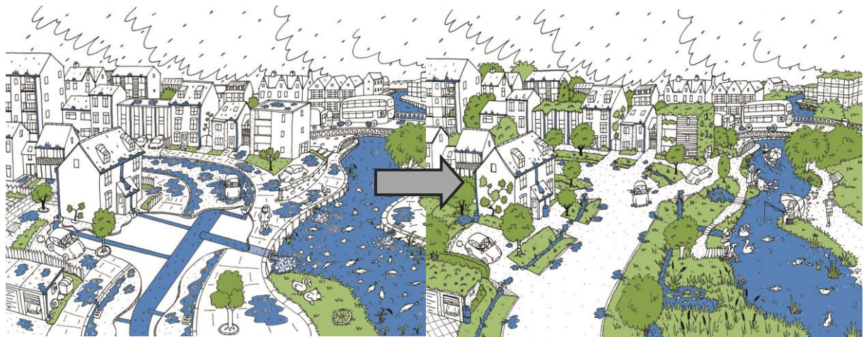
Figure 2.4- Illustration demonstrating the implementation of SUDS, replicating natural pre-development drainage as much as possible. Source: Thames21@ (2020).
