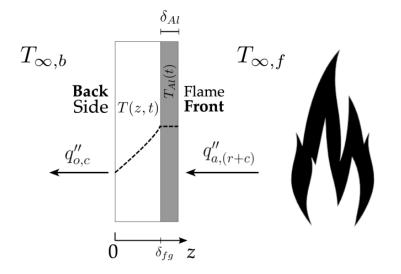
Figure 2.1: Schematic of the fiberglass coated with aluminum.
