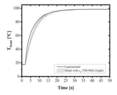
Figure 4.3: Front temperature evolution of the barrier.
