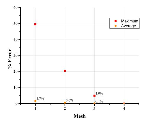
Figure 2.4: Average error and maximum error percentage evolution relative to mesh 4 (For Bi = 1,  $C_{t,f}^* = 0.5$  and  $\phi_h = 100^{\circ}C$ ).
