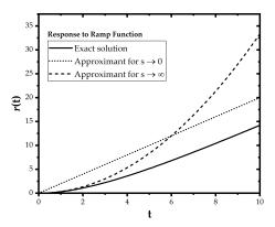
Figure 3: Response to a ramp input function (slope=1) for all transfer functions (For K=2 and  $\tau = 3$ ).
