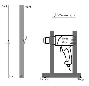
Figure 3.1: Illustration of the experimental setup built to validate the heat transfer model.
