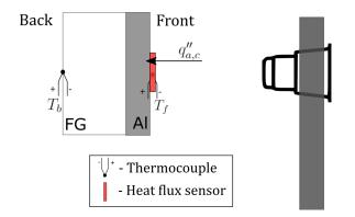
Figure 3.2: Experimental Setup to determine  $k_{fg}$
