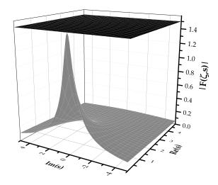
Figure 2.2: Exact transfer function (gray) and steady-state transfer function (black) (For Bi = 1,  $C_{t,f}^* = 0.5$  and  $\zeta = 0.5$ ).
