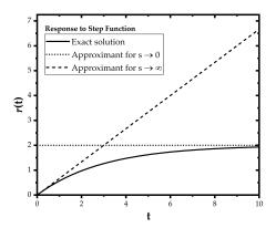
Figure 2: Response to a unitary step input function for all transfer functions (For K=2 and  $\tau = 3$ ).
