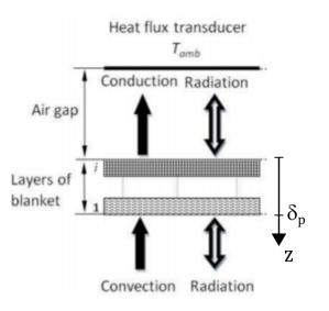
Figure 1.7: Fire blanket model by Hsu et al. (2011).
