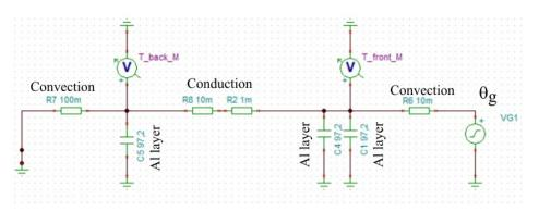
Figure 4.9: System M electrical analog.
