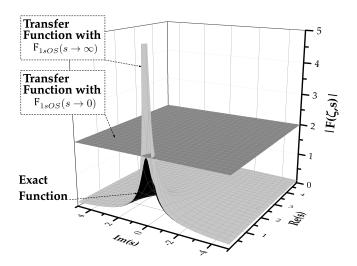
**Figure 1:** Exact transfer function (black),  $F_{1sOS}(s \to 0)$  transfer function (dark grey) and  $F_{1sOS}(s \to \infty)$  transfer function (light grey) (For K = 2 and  $\tau = 3$ ).
