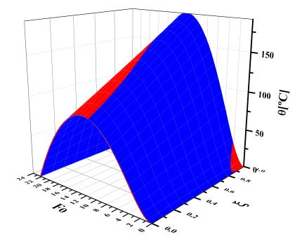
Figure 2.6: Approximate solution (blue) and reference solution (red) (For Fo<sub>max</sub> = 10, Bi = 1 and  $C_{t,f}^* = 0.5$ ).
