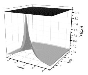
Figure 2.3: Exact transfer function (dark grey), Approximate function (light grey) and Quasi-static function (black) (For Bi = 1,  $C_{t,f}^* = 0.5$  and  $\zeta = 0.5$ ).
