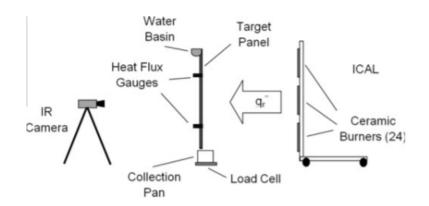
Figure 1.4: Experimental setup used by Meredith et al. (2013)
