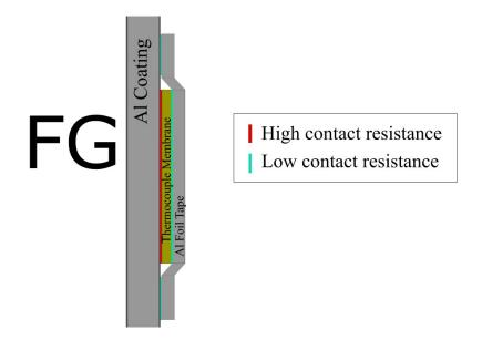
Figure 4.8: Simplified representation of the thermocouple installation.
