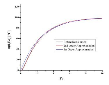
Figure 2.8: 1st order Approximate solution (blue), 2nd order Approximate solution (red) and reference solution (black) (For Bi = 1,  $C_{t,f}^* = 0.5$  and  $\phi_h = 100^{\circ}C$ ).
