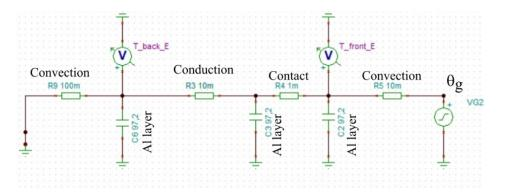
Figure 4.10: System E electrical analog.
