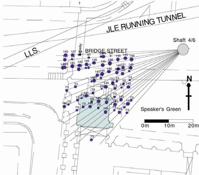
Figure 11- Top view of compensation grouting carried out underneath Big Ben during the construction of the Jubilee Line Extension (Harris et al., 1999).
