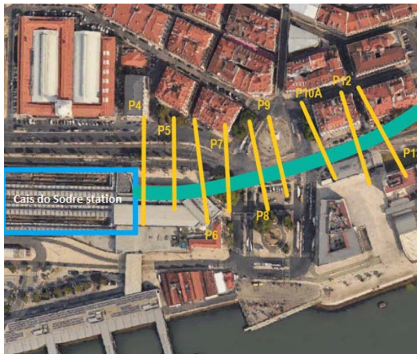
Figure 26- Top view from the instrumentation survey from sections P4 to P13 of section 63 in 0+200m to 0+500m between Cais do Sodre station – Baixa/Chiado station.
