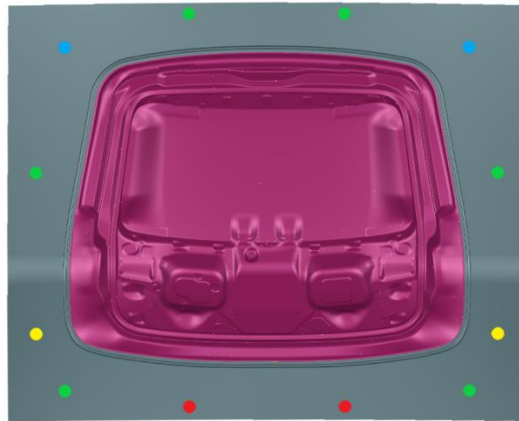
Figure 5.16. Position of the cylinders in the upper blankholder and corresponding sets defined by color.
