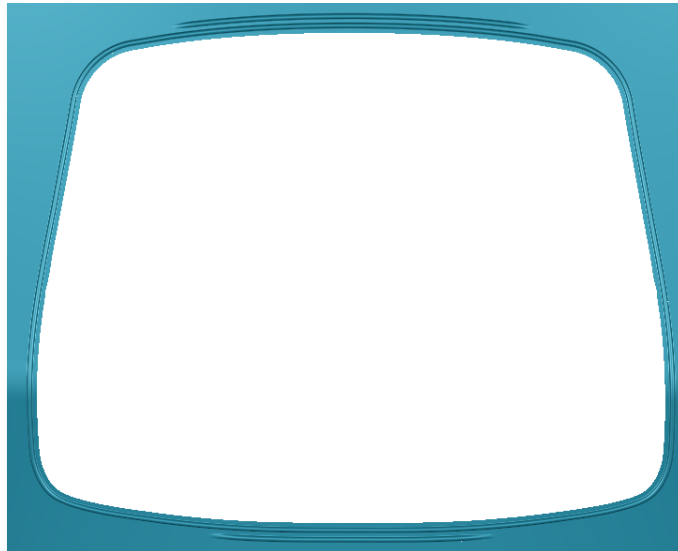
Figure 5.29. Additional drawbeads, in the lower and upper part of the upper blankholder.
