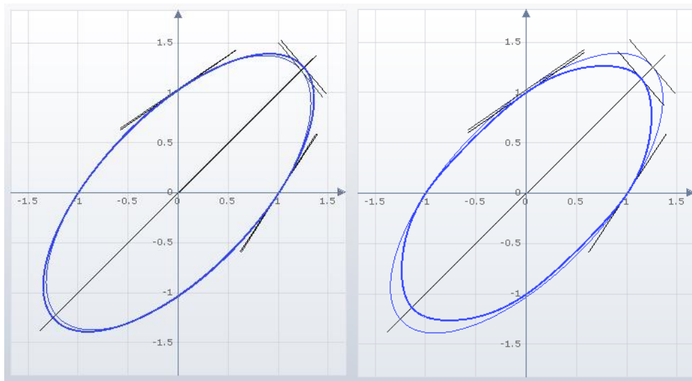
Figure 5.26. Left: Normalized Hill'48 yield curves for the material properties from the library (fine line) and from the tensile tests data (thick line). Right: Normalized yield curves obtained from tensile test data for Hill'48 (fine line) and Vegter 2017 (thick line).
