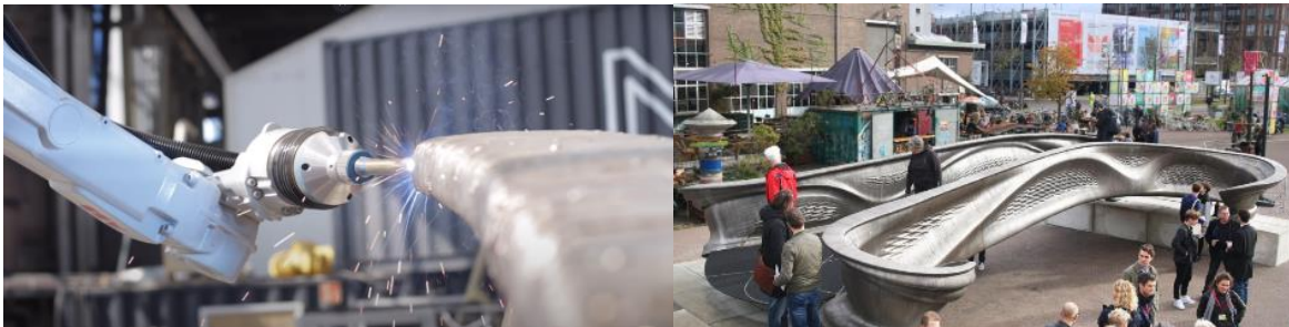
Figure 10- Horizontal print of MX3D Bridge. (MX3D Bridge | MX3D)
