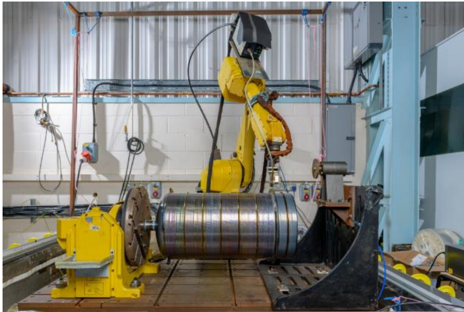
Figure 4- Manufacturing of Thales Alenia's pressure vessel. (Titanium pressure vessel for space exploration built successfully using the Wire + Arc Additive Manufacturing process 2017)
