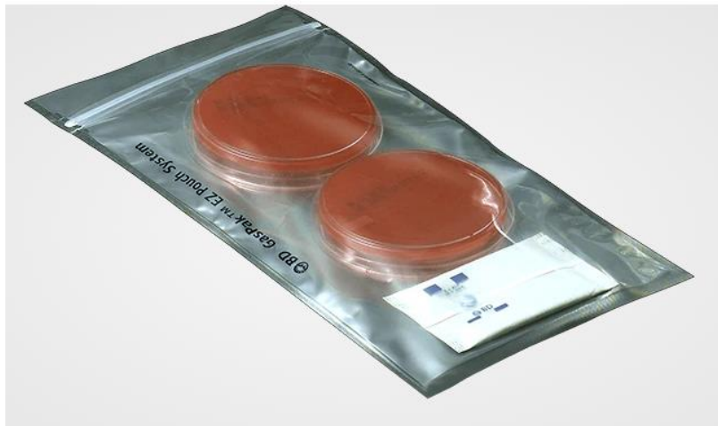
Figure 2.1 – BD GasPak EZ Anaerobe Pouch System with the Indicator, containing two cell dishes.
