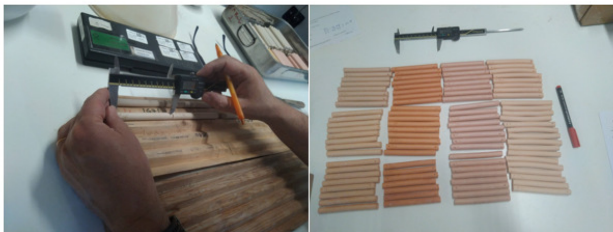
Figure V. 4 Measuring the retraction at sample pieces after dried and fired
