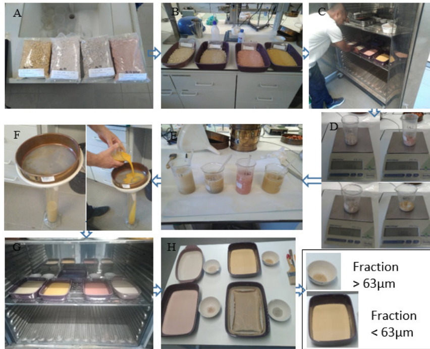
Figure IV. 5 (A) Preparation of 500g for each sample to granulometric analysis (B and C) Preparation and drying in a dryer at 110°C for 24 hours (D) Weighing 50 g of 500 g for each sample (E) Mixed with 200 ml hexametaphosphate liquid and then shaken and leave it for 24 hours (F) Determination of residuals; Fraction<63µm and fraction>63 µm separated on a wet sieve (G) Dried residuals material (fraction<63 µm and fraction>63 µm) in a dryer at 110°C for 24 hours (H) Two samples (fraction<63 µm and fraction>63 µm) prepared for granulometric analysis.
