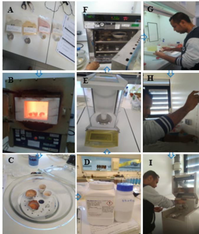
Figure IV. 4 (A) Samples sieved at 200 mesh ASTM (75 \mu m) (B) The sample to be dried at 1000 \pm 100 °C for 1 hour (C) Put and allow to cool in a desiccator to room temperature (D) Spectroflux 110, lithium tetraborate (E) Weigh 10 grams of spectroflux 110, lithium tetraborate (F) Dried Spectroflux 110, lithium tetraborate at 100-110 °C (G) Mixture kaolin sample with lithium tertaborate (H) Add to the mixture about 1 ml of lithium bromide in 5% solution (I) Equipment Call Per'X 3 (IT 311.017) to prepare samples like pearl cup for chemical analysis.
