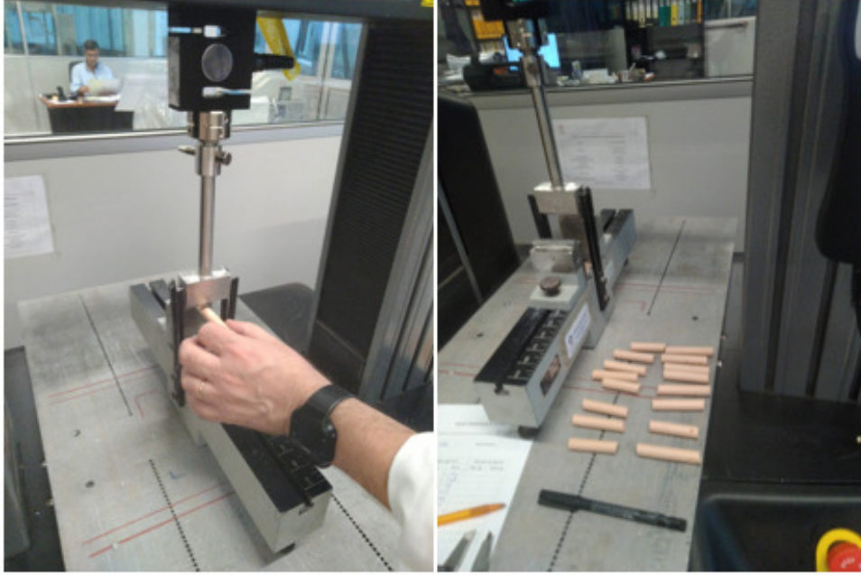
Figure V. 6 MFS testing process on sample pieces at different temperatures (dried and after firing).
