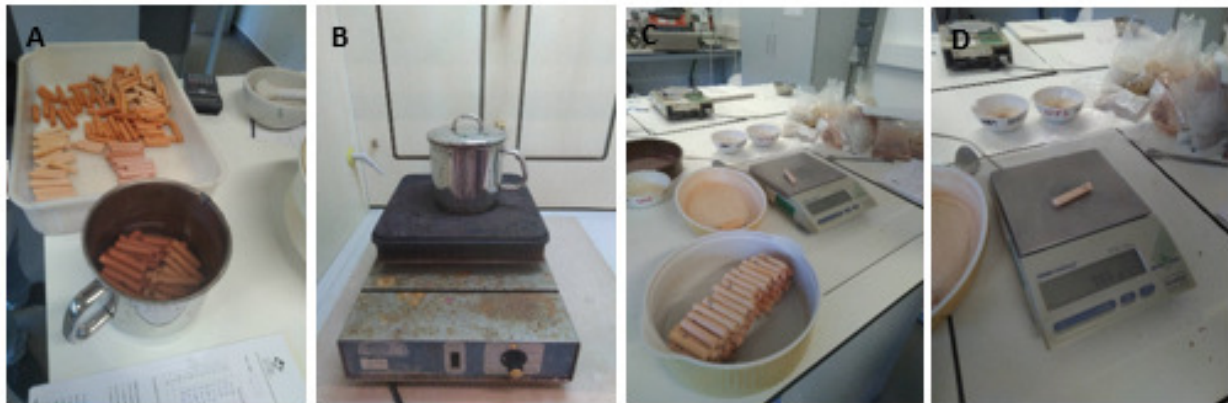
Figure IV. 9 (A) sample that has been fired at different temperatures of 110 °C, 850 °C, 950 °C and 1050C; (C, B) Determination of water absorption in firing specimens; (C, D) Weighing each specimen before and after it is fired.
