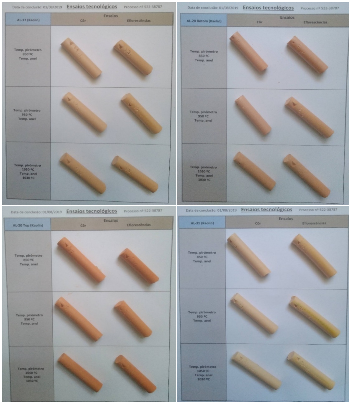
Figure V. 10 Results of color and efflorescence after drying and firing the sample pieces at different temperatures.
