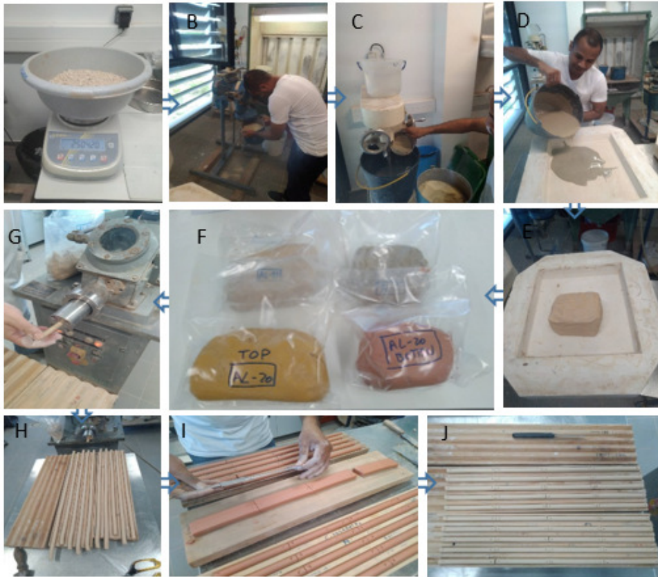
Figure IV. 6 (A) Weigh 250g of kaolin sample (B) Hammer mill as equipment tool to reduce the sample size (C) Shaker tool for stirring water (2 liters) with kaolin (250g) (D) Drainage of water on the kaolin sample with gypsum tube (E and F) kaolin in a moist state in the gypsum tube and ready to be formed into specimens (G) “Planetary mill” tool is used to make specimen samples for technological tests (H, I and J) Specimen sample results; 40 specimens are required for each sample.
