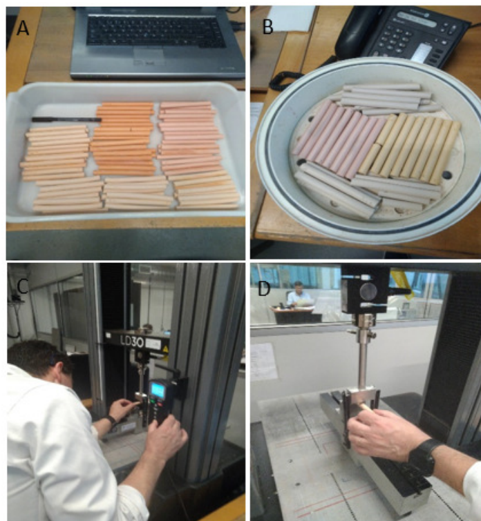
Figure IV.8 (A and B) Samples that have been dried (110 °C ) and fired at different temperatures (850 °C, 950 °C and 1050 °C); (C, D) Mechanical flexural strength (MFS) test.
