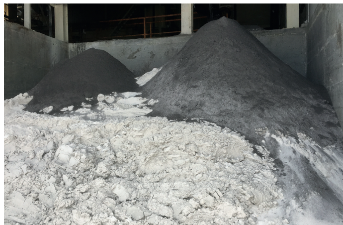
Figure 3.13. Rejected material concentrated in heavy minerals.
