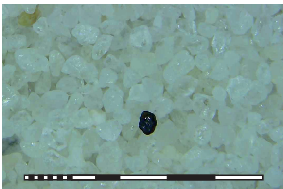
Figure 4.17. S40/45 FL Line 2 sand. Scale is 5 mm.
