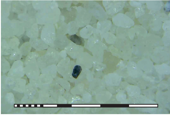
Figure 4.3. S40 sand. Scale is 5 mm.
