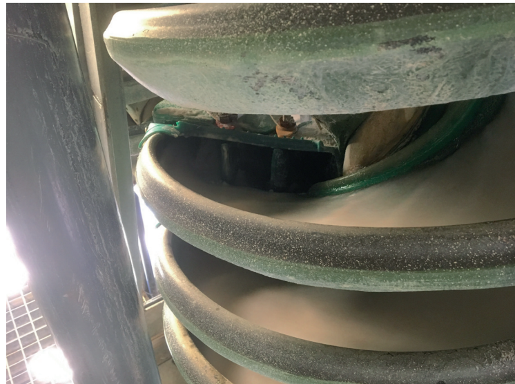
Figure 3.11. Inside of spirals showing separation outlets.
