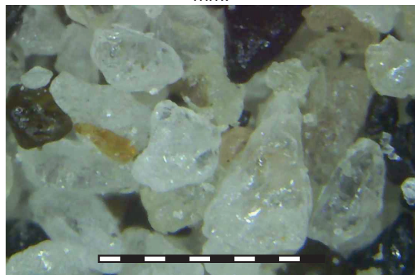
Figure 4.14. Line 2 rejected sand. Scale is 1 mm.
