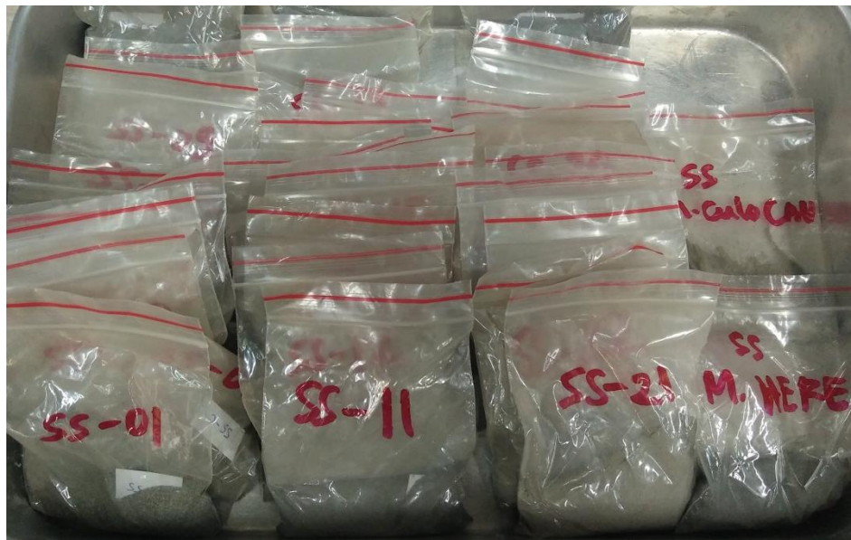
Figure 3.3 Fine Fractions < 180 microns about 150-200g in plastic bags after decanted excess water.
