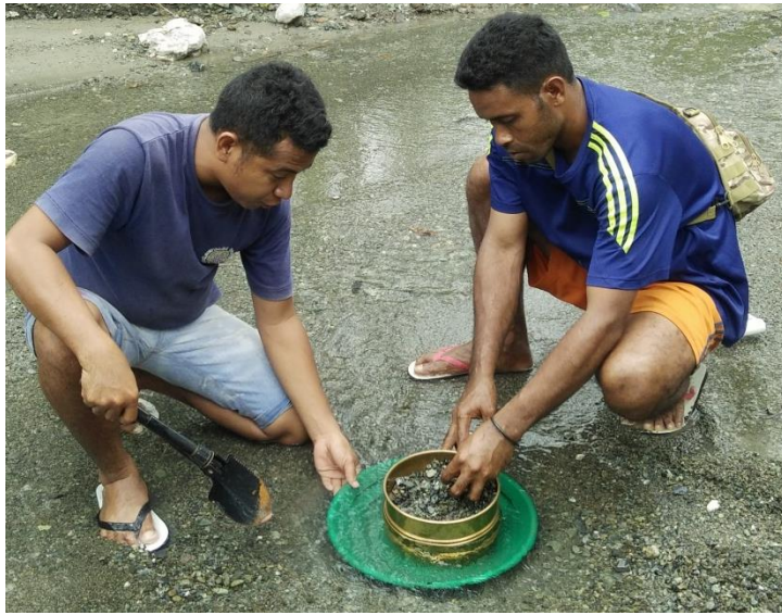
Figure 3.2. The sieve of 2mm was placed on the top of the fine sieve (180 \mu m) and both were mounted on the top of the pan.
