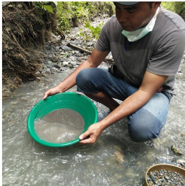
Figure 3.4. Sieve the sediments on screen, remove the large clastic and rub the material to promote disaggregation
