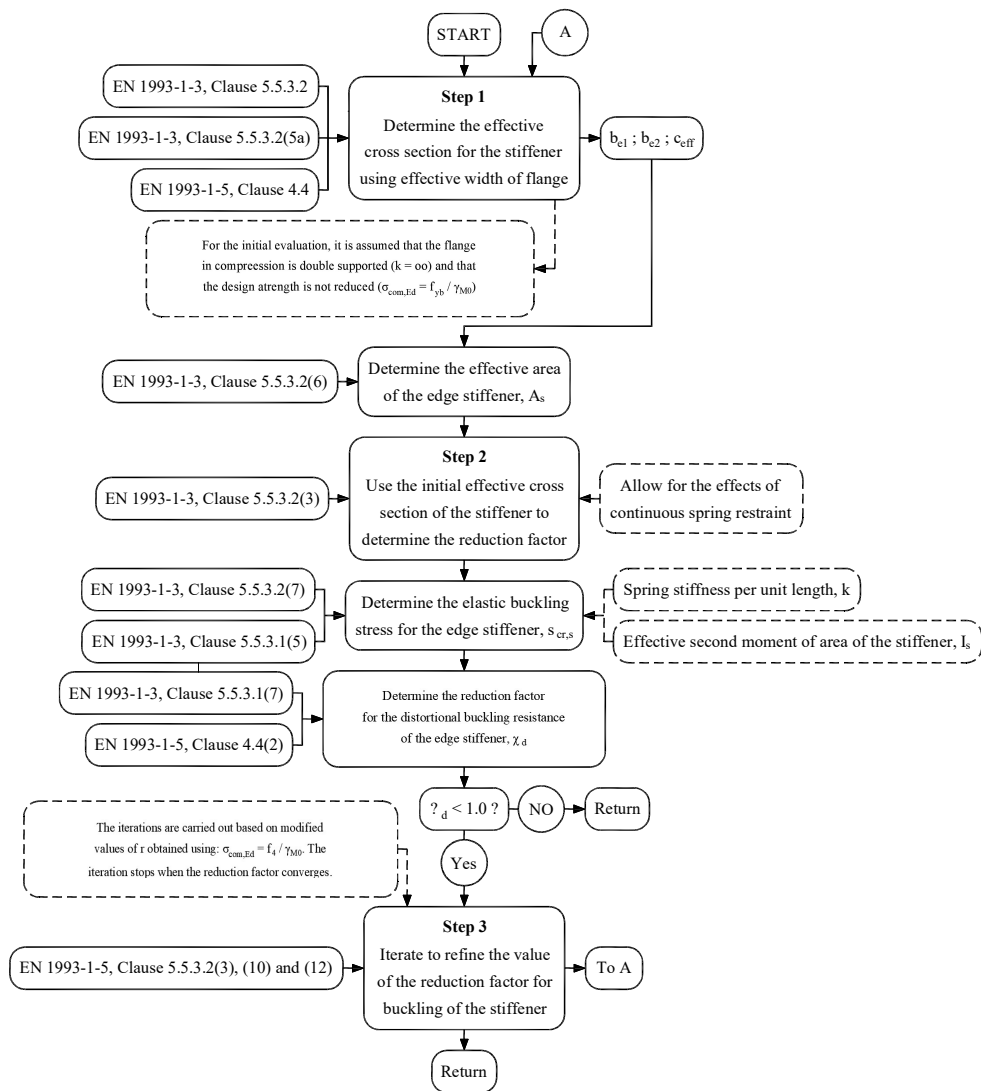
Figure 4.8 - Flow Chart: Calculation of effective section properties of the flange and lip in compression - General iterative procedure (Adapted from SF038a-EN-EU, 2006)
