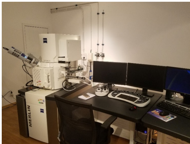
Figure 6: The SEM instrument equipped with WDS detector used for studying morphology and chemical composition of samples.
