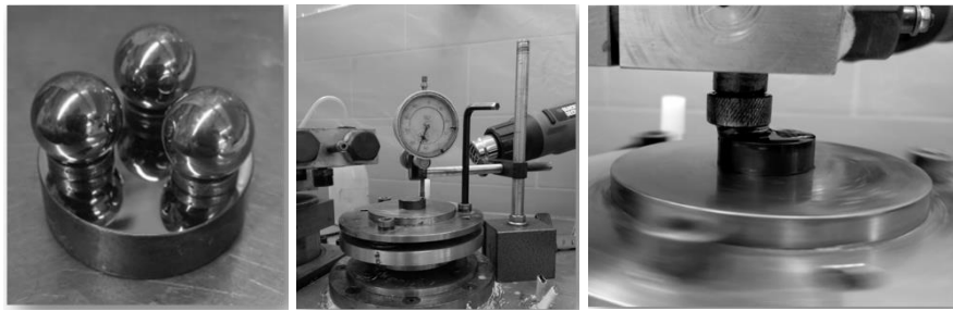
Figure 4.2. (a) Polished rings and disc. (b) Alignment process. (c) Test set-up.
