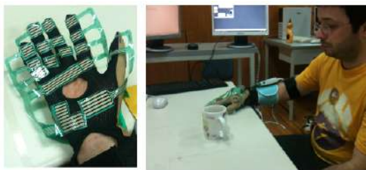
Fig. 4. On the left: Configuration of the tactile sensing array on the hand surface. On the Right: Configuration of the experimental area.
