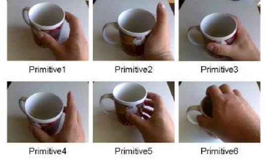
Fig. 3. Representation of six of the pre-defined grasp configurations used to estimate the corresponding static contact state templates.
