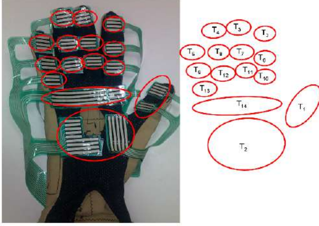
Fig. 2. Representation of the 15 tactile sensing regions defined from the 360 sensing elements of the tactile sensing device.
