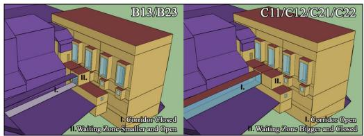
**Figure 2**. Northern façade with: (a) a smaller Waiting Zone and openly connected to the Noble Floor & the Corridor is exterior; or (b) a bigger and closed Waiting Zone & the Corridor is closed.
