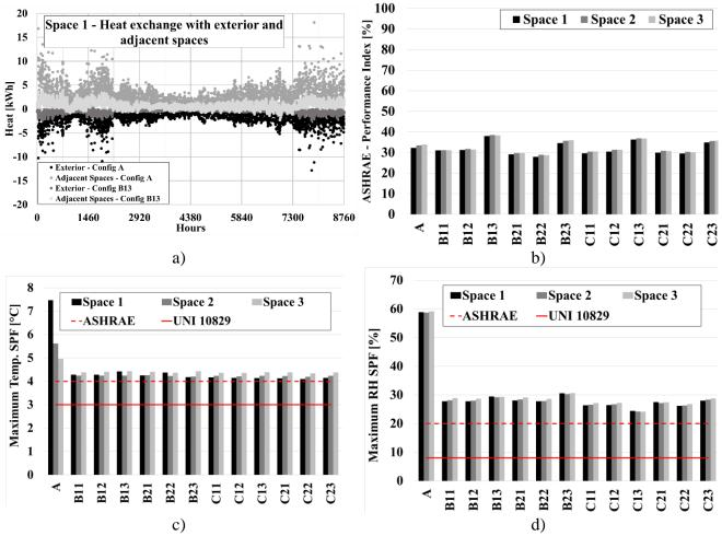
**Figure 3.** (a) Heat exchanges of Space 1 with exterior and adjacent spaces (config. A: black and normal grey; config. B13: dark and light grey); (b) PI according to ASHRAE; (c) annual maximum values for temperature SPF (d) annual maximum values for relative humidity SPF.
