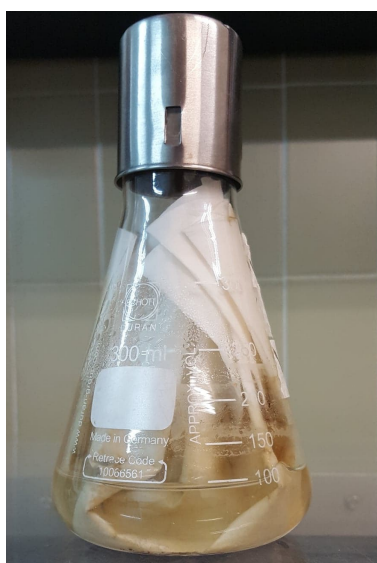
Figure 7. Example of an Erlenmeyer with 1g of Panasqueira mine tailings and a paper filter acting as a physical membrane between the bacterial cells and the mine tailings.
