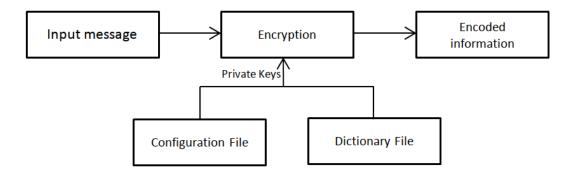
Figure 3.5: Developed cryptosystem with the separate private keys.
