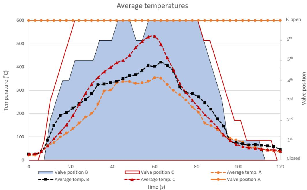
**Figure 4.14** – Average temperature and valve position for each test
