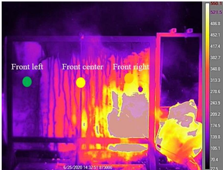
**Figure 4.5** – Fabric temperature distribution at  $t=66s$  during the first experiment
