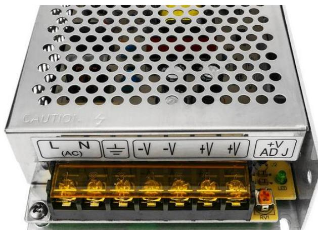
Figure 2.9 – Power supply used, showing its connections
