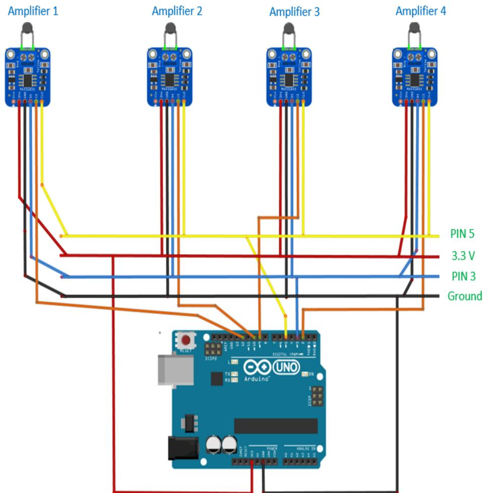
**Figure 2.12** – Detail of the wiring scheme between the Arduino® and the four thermocouple amplifiers.
