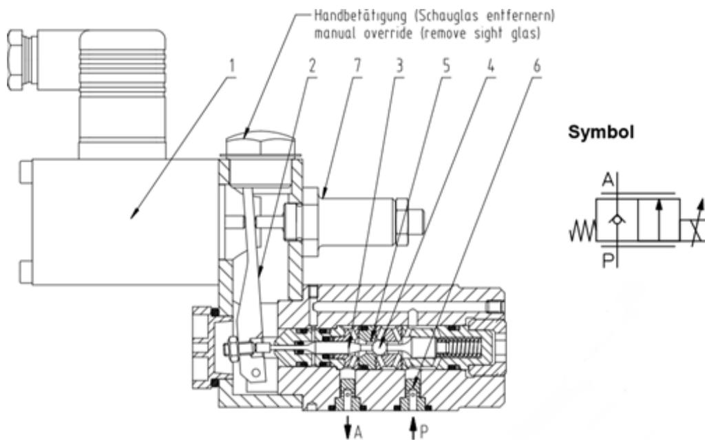
Figure 2.3 – Valve operating scheme
