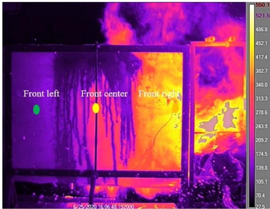
**Figure 4.9** – Fabric temperature distribution at t=66s during the second experiment
