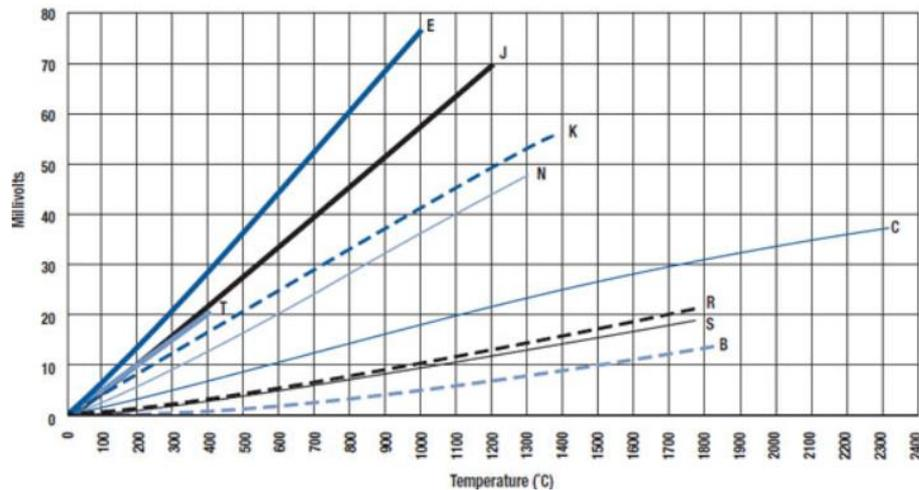
Figure 2.10 – Response of the different types of thermocouples
