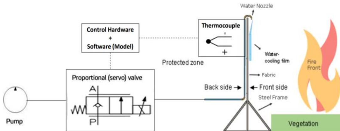
Figure 2.1 – Barrier with water distribution control system, (Viegas, et al., 2019)
