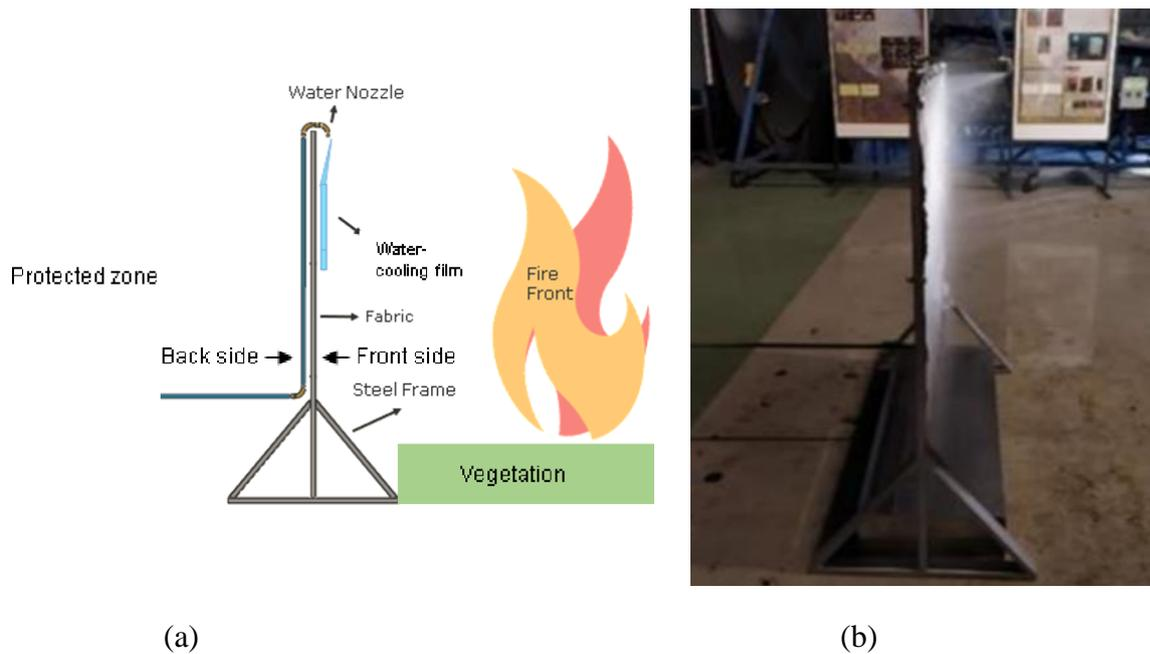
**Figure 1.6** – (a) Barrier scheme (b) Barrier prototype in action, (Viegas, et al., 2019)
