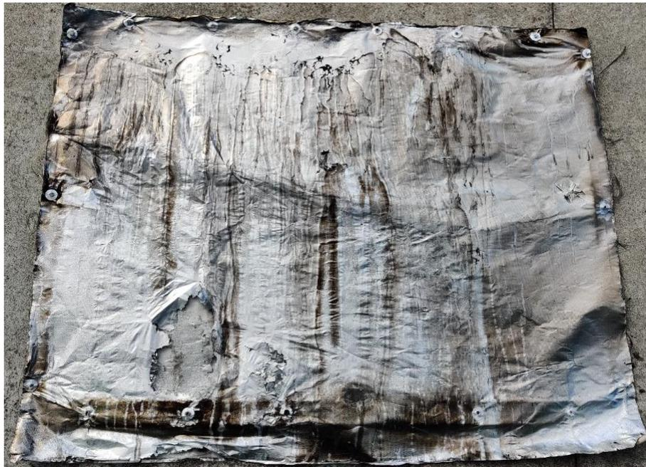
**Figure 4.13** –The fire barrier fabric after the first experiment
