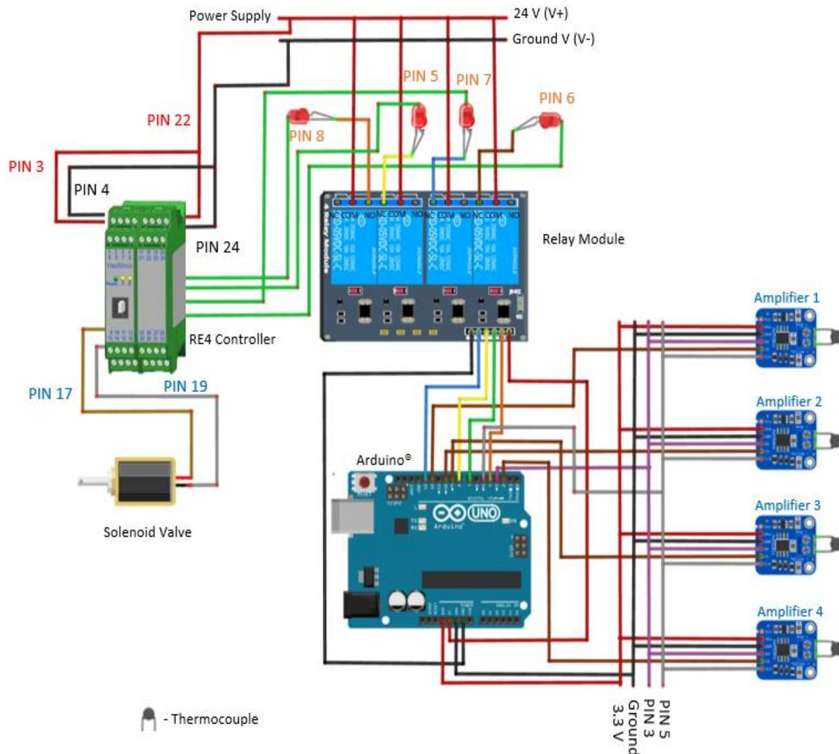
**Figure 2.2** – Wiring scheme for proposed closed-loop control
