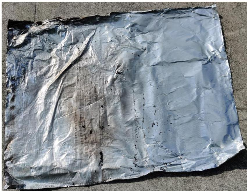
**Figure 4.10** – The fire barrier fabric after the second experiment
