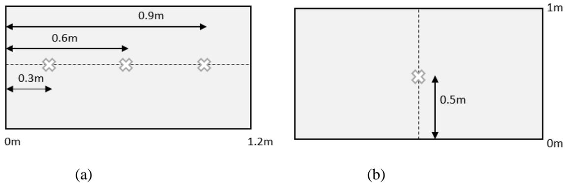
**Figure 4.2** – Thermocouples distribution in (a) front of the barrier (b) back of the barrier
