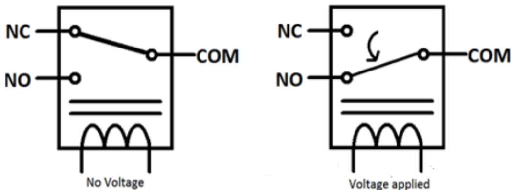
Figure 2.7 – Representative scheme of the relay operation
