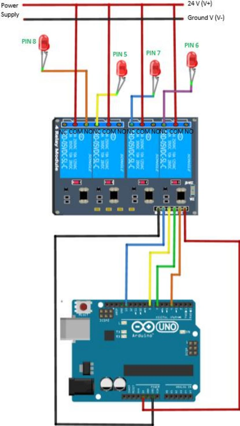
Figure 2.8 – Scheme of the connection between Arduino® and controller via relays
