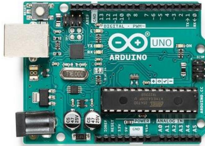
Figure 2.6 – Arduino® Uno Rev 3 board
