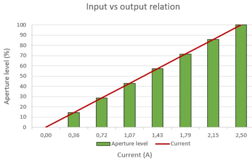
**Figure 3.3** – Response curve of the valve solenoid according to the input signal current
