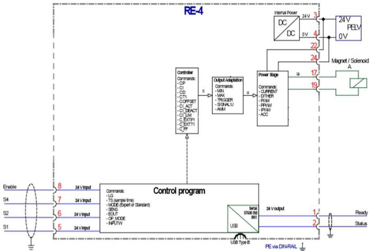
Figure 2.5 – Operation diagram of the RE4 controller, Hauinco manual
