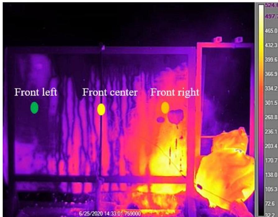
**Figure 4.7** – Fabric temperature distribution at  $t=75s$  during the first experiment
