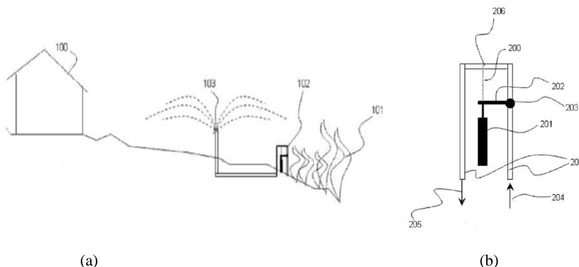
**Figure 1.2** – (a) Basic scheme of Yount’s mechanism; (b) Hair trigger mechanism in detail
