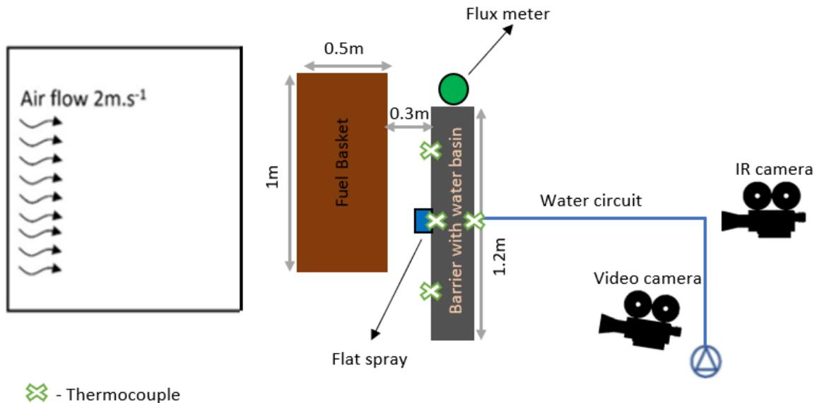
**Figure 4.1** – Representation of the experimental assembly
