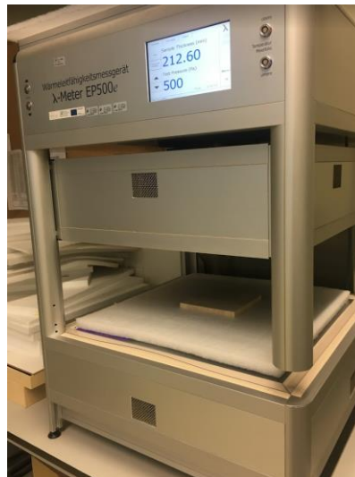
Figure B.2. Confinement of balsa wood specimen with an insulation material.
