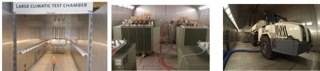
Figure 2.8. High performance and large-scale examples of climatic chambers for testing. Sirris (2020).
