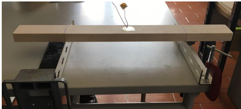
Figure 4.6. IET test configuration for bigger specimen's dimensions.
