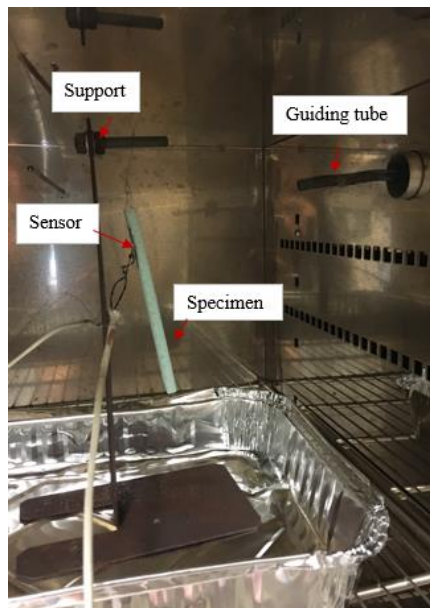
Figure 4.1. IET test configuration.
