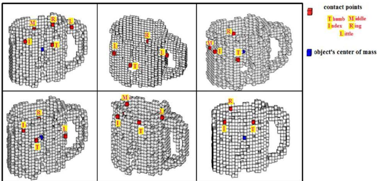
**Fig. 19.** Sequence of some contact points overlaid in the static representation of the object (volumetric map) during the manipulation task. The contact points are given by the fingertips locations during the in-hand manipulation phase.
