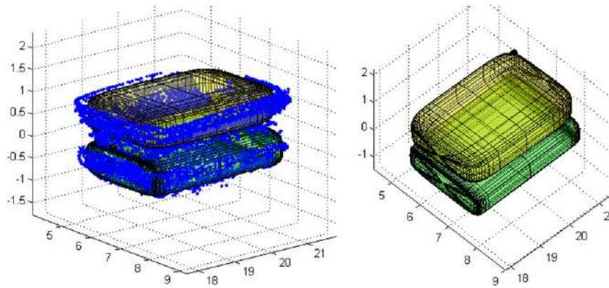
**Fig. 16.** Object (sponge) shape approximation using superquadrics after the segmentation process shown in Fig. 14. Left image shows the superquadrics on the 3D points cloud of the computed probabilistic map and (b) are the superquadrics (boxes) generated for this object.
