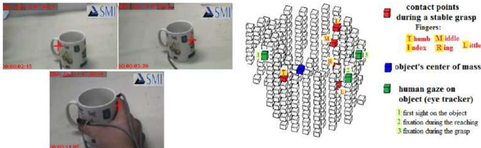
**Fig. 13.** Human gaze during grasping and the contact points on the object surface. Task: Reaching and Grasping the mug by side-grasp. This type of grasping was chosen due to the orientation of the object – it influences the type of grasping.
