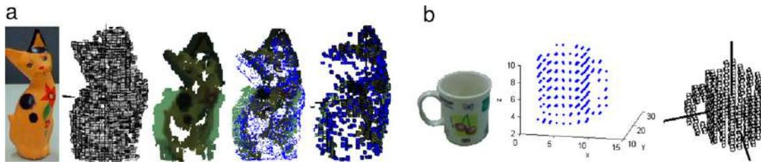
**Fig. 10.** Probabilistic representation of objects derived from in-hand exploration. (a) A wooden cat; computed probabilistic map; visual information (textured points cloud); probabilistic map with texture information (only voxels with probability higher than 0.8). (b) Image of a mug following the view of the occupied voxel's central points, and the last image shows the computed map derived from in-hand exploration (object-centred representation).
