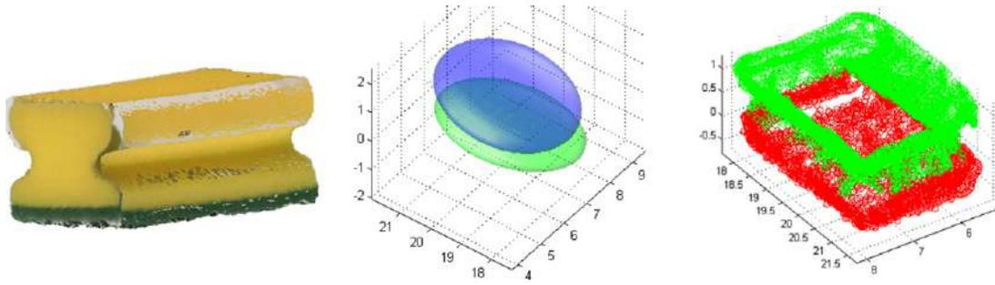
**Fig. 14.** Object segmentation of a sponge with the method proposed, using  $K_{\max} = 2$  and 3D points acquired by in-hand exploration of the object surface. On the left is an image of the object; in the middle the 2 clusters (Gaussian density functions) obtained from the segmentation process; and on the right the colour labelled 3D points of the segmented clusters.
