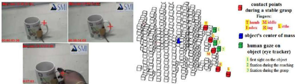
**Fig. 12.** Human gaze during grasping and the contact points on the object surface. Task: Reaching and Grasping by the Object Handle. The visual gaze during the grasping shows that the human usually looks to the region of the object where will be performed the grasp.
