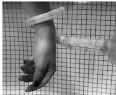
Figure 2.4. Octopus robot arm with cables and SMAs springs [4].
