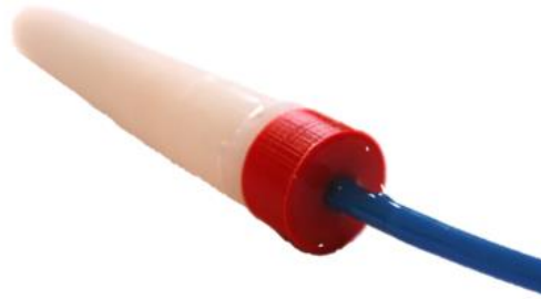
Figure 4.11. Fibre-reinforced index actuator.
