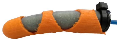
Figure 4.4. Assembly of the finger exoskeleton and the fibre-reinforced actuator.
