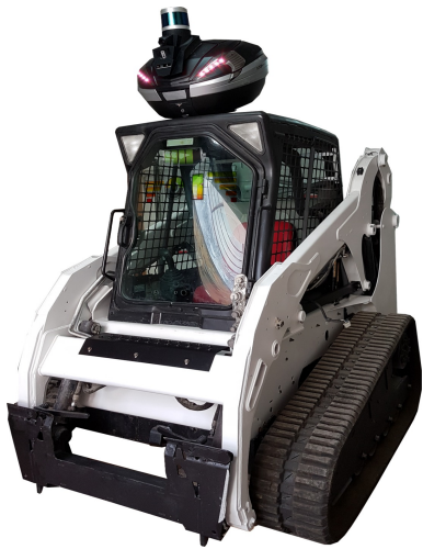
(a) Ranger platform without the mechanical mulcher attachment.
