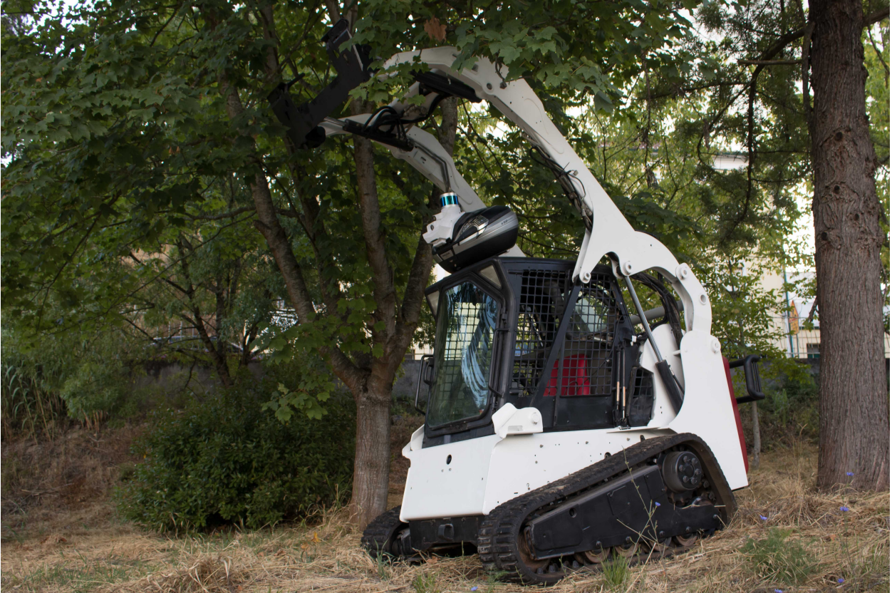
Figure 1.1: The Ranger UGV being teleoperated in a realistic test in a forest environment. Its main sensors can be seen in its head, see Section 4.1.1 for more details.
