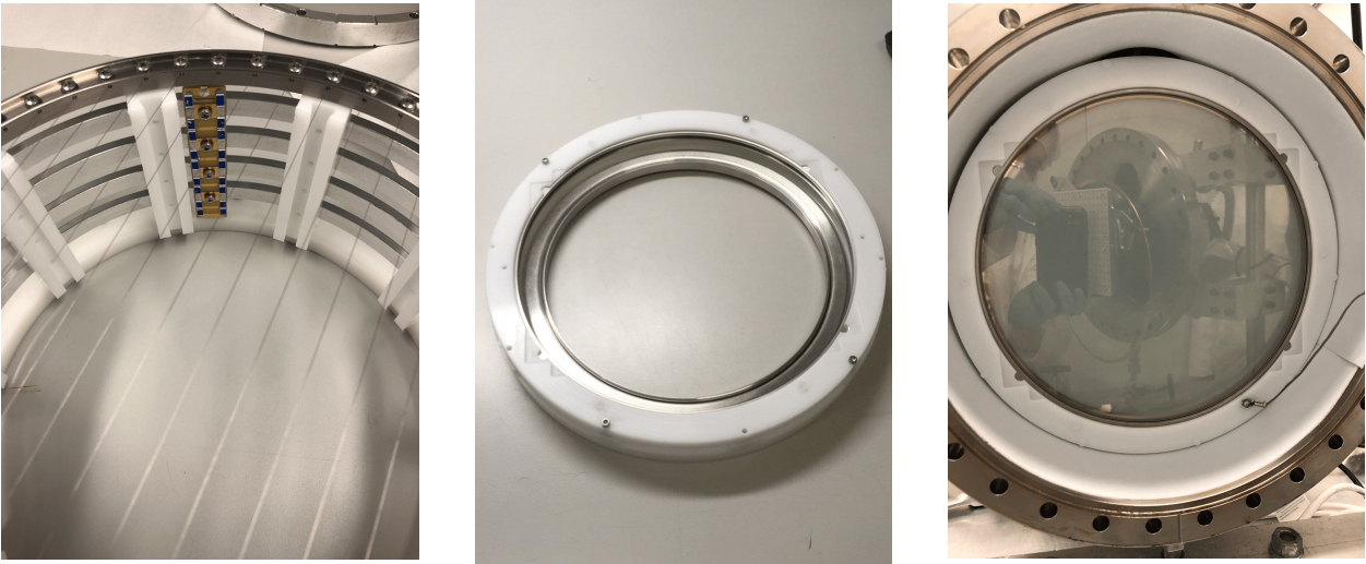
Figure 4.6: Closer look of the cathode grid (left), gate mesh (center) and the anode glass plate (right).
