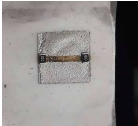
Figure 3.10: Sample used in SEM analysis for the interface characterization. In this case, 2 resistors were interfaced with the ink over the gap created with the laser. The samples were then cropped over the ink close to the interface to produce small specimens with individual components.
