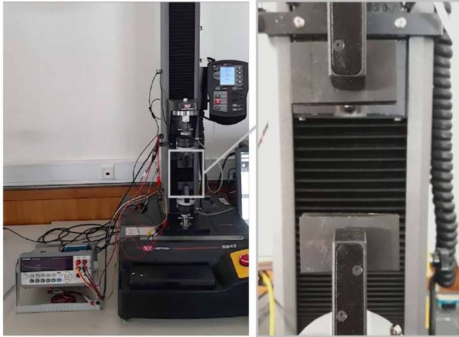
Figure 3.6: Equipment used in the electromechanical characterization tests. INSTRON 5900 and supporting multimeter used in the tests and closeup of the grips of the INSTRON machine where the sample is immobilized and stretched.
