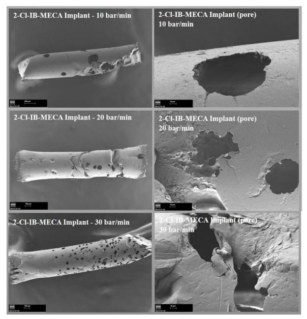
Figure 16 - After release SEM images of 2-Cl-IB-MECA implants.
