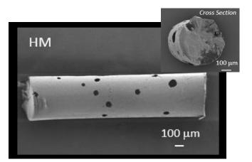
Figure 7 - SEM: implant prepared by hot melting.
