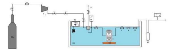
Figure B1 – Schematic diagram of the supercritical solvent unit. C1: compressor; TC: temperature controller; WB: water bath; P: purge; PT: pressure transducer; S: sample; MS: magnetic stirrer; C: high pressure vessel; V: screw down valve; M: macrometric valve; m: micrometric valve; GT: glass trap; F: mass flow meter (Rosa, 2013).
