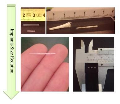
Figure 2 - Evolution of Implants Size Reduction during investigation.
