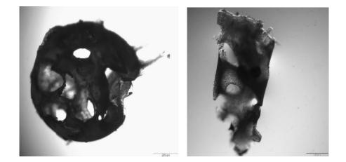
Figure 5 - Optical Microscope image of 8% (w/w) glycofurol in PCL implant: initial tests. Implants were totally removed from catheter tube and have porosity.
