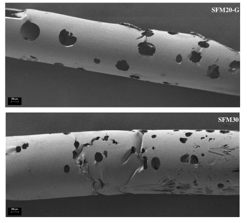
Figure 6 - SEM: implants prepared by scCO<sub>2</sub> foaming process for 2h, 20 MPa, 45°C. Depressurization rates were variable. At depressurization rate of 20 bar/min, samples with and without Glycofurol were analyzed.
