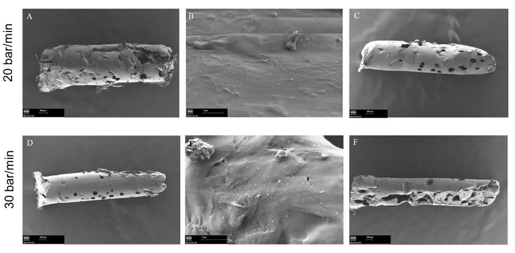
Figure 17 - 2-Cl-IB-MECA implants SEM images before and after release with body and surface details.
