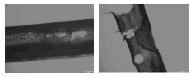
Figure 4 - Optical Microscope images of 22% (w/w) glycofurol in PCL implant: catheter walls that could not be removed in its entirety and large pores of the implant are visible.
