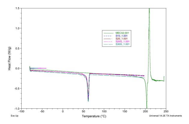
Figure 10 - Samples thermal analysis: DSC thermograms.
