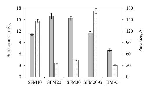
Figure 8 - Implants surface area and pore size in different processing conditions: ■ surface area □ pore size
