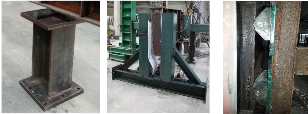
Figure 3.7 - Support conditions beam tests: a) intermediate support; b) Lateral restraint at the free end; c) Lateral restraint at the intermediate support
