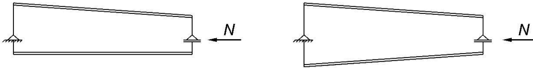
Figure 3.1– a) “L”-shape tapered member; b) “V”-shape tapered member
