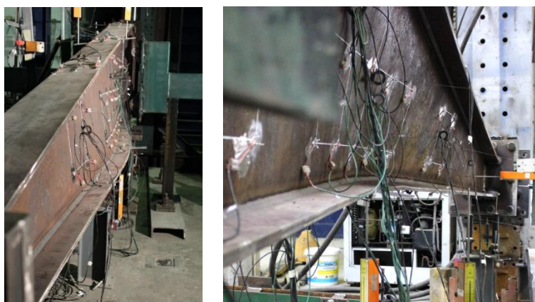
Figure 3.35 - Collapse mode of test B1
