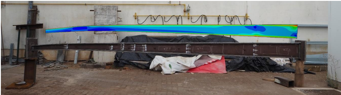
Figure 4.12 Column 3: numerical and experimental deformed shape
