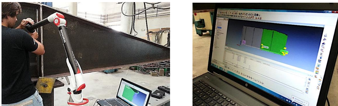
Figure 3.11 - Geometrical imperfections: a) Laser system used; b) 3D model
