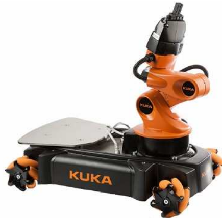
Figure 2-7 – KUKA youBot platform for scientists and researchers [30].
