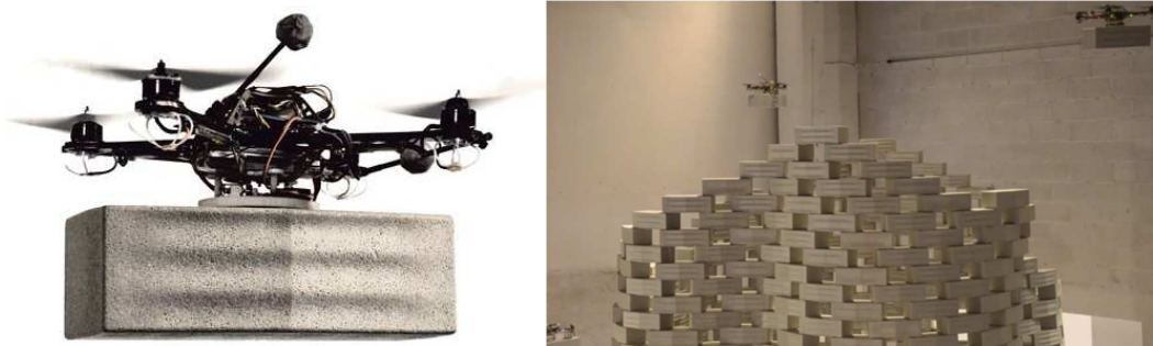
Figure 2-13 – Air Drones from ETH Zürich's Institute for Dynamic Systems and Control building a 6 meter tall tower, autonomously[41].
