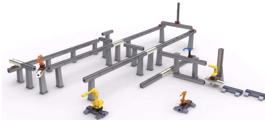
Figure 2-17 - Lucas Robotics System relying on motorized 3D scaffold[51].
