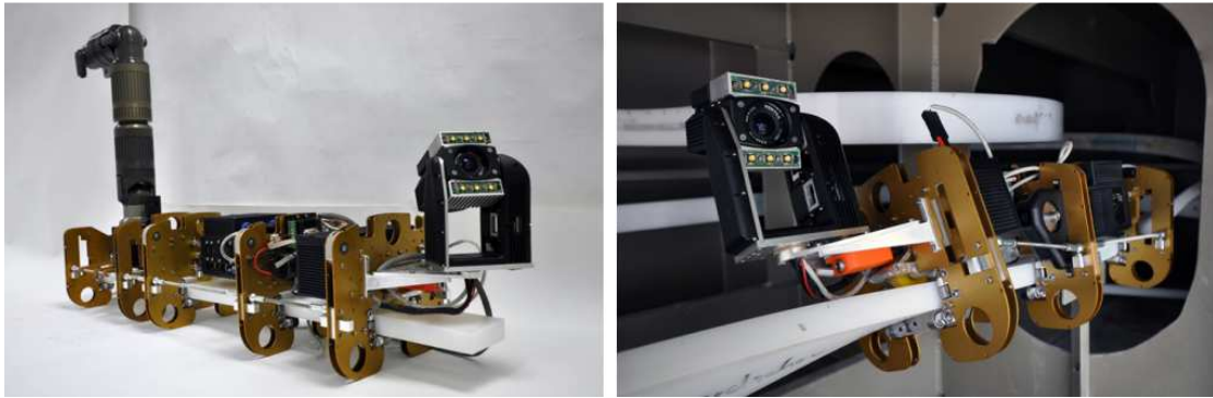
Figure 2-15 - ARTIS robot with 5 modules and manipulator arm, and the robot moving on a rail[47].
