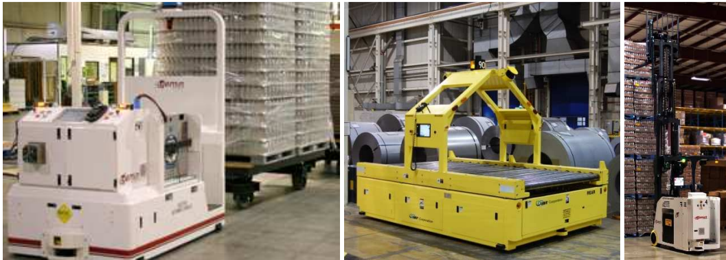
Figure 2-3 – Few examples of different AGV types. From left to right, towing vehicle [25], load transfer vehicle[26] and forklift vehicle[27].
