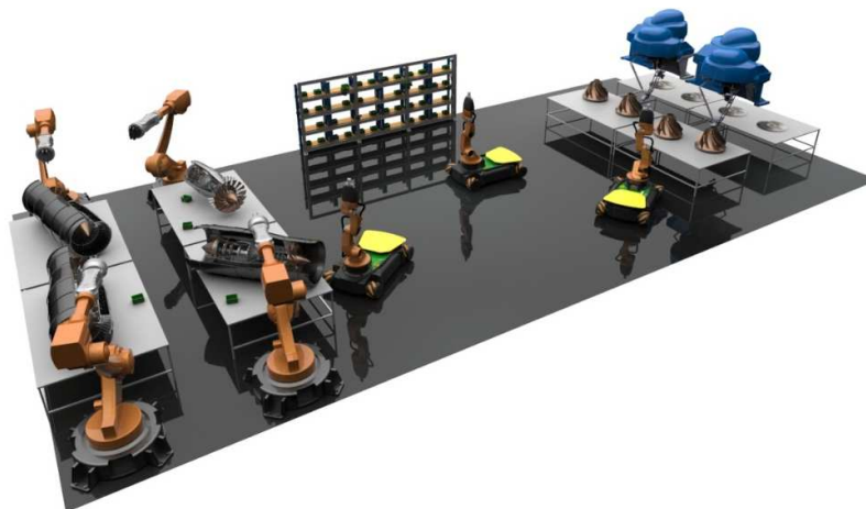
Figure 4-38 – Comparable setup using existing automation solutions: 4 robotic arms, 4 delta 3D printers and 3 AGV's equipped with a robot arm.
