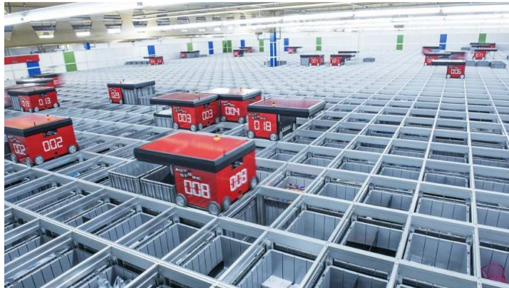
Figure 2-19 – The Autostore warehouse automation system moving on passive 2D horizontal grid of rails[54].
