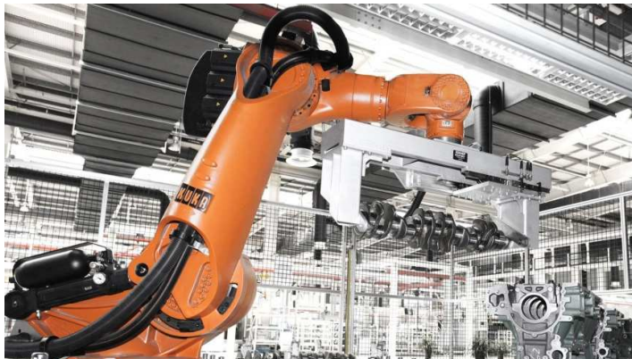
Figure 2-1 - The KUKA KR 1000 titan handling a crankshaft in a heavy-duty diesel engine factory[21].
