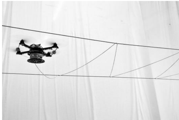
Figure 2-14 – Air Drone making a cable-net structure[43].
