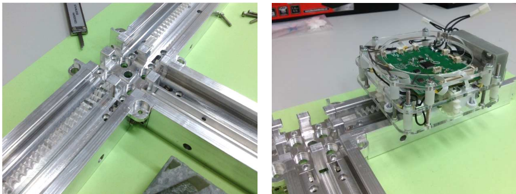
Figure 4-4 – SCALA generation TWO prototype, showing the mobile agent and custom made rails and junction, made in a CNC machine.
