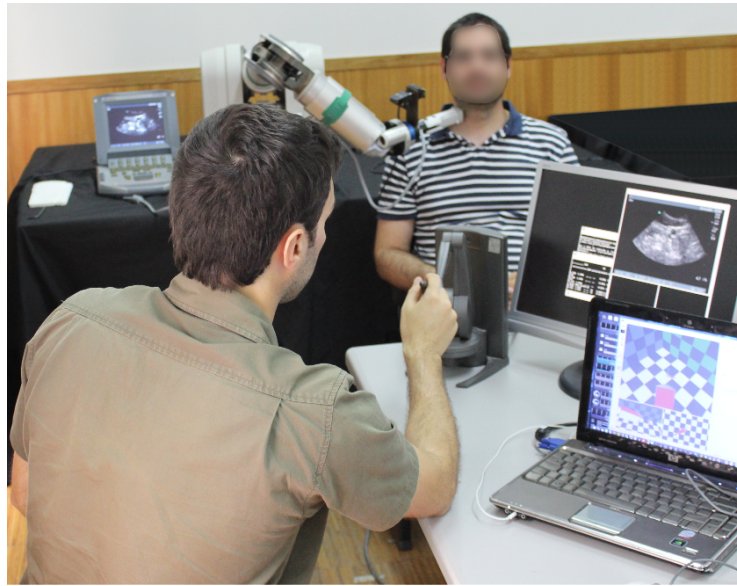
Figure 2.4— Robotic-assisted tele-echography system in a local setup. Illustrative example.
