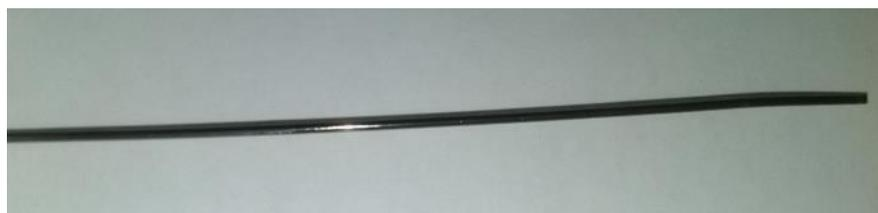
**Figura 2.1** Fio de Nitinol,  $\phi = 0,70$  mm.
