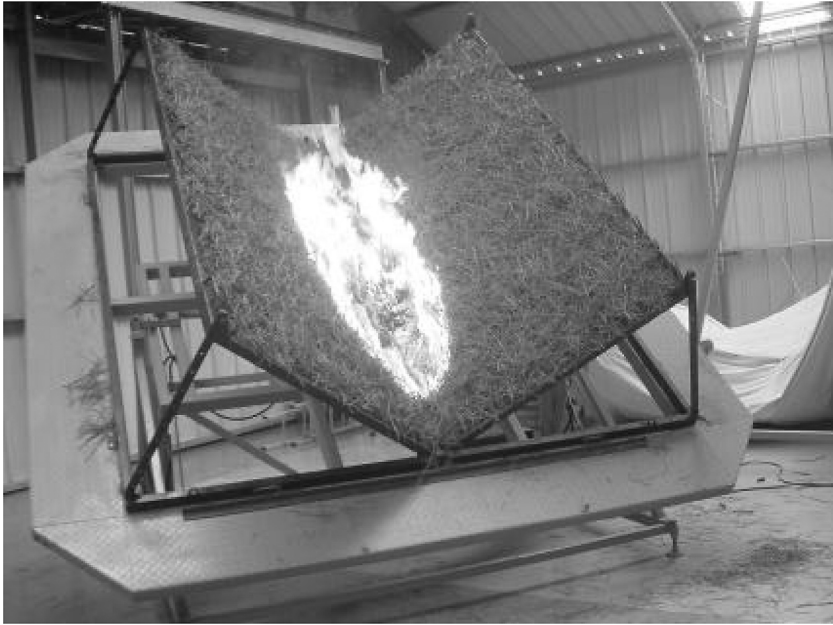
Figure 1. Experimental setup in the Forest Fire Laboratory of the University of Coimbra for the study of fire spread in canyons and for the observation and analysis of blowup phenomena.
