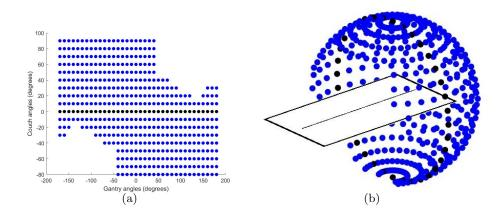
**Fig. 1.** Candidate beams homogeneously distributed represented in 2D - 1(a) and the corresponding 3D representation -1(b). Black beams correspond to the coplanar candidate beams (couch fixed at  $0^{\circ}$ ) while blue beams correspond to noncoplanar candidate beams.
