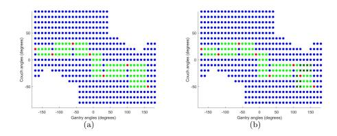
**Fig. 2.** The 7-beam noncoplanar BAO solution is displayed in red and the feasible points to consider when calculating a new anchor point are displayed in green -2(a). A novel anchor point is added and green candidate beams that became infeasible are removed -2(b).
