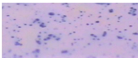
Figure 2.20. Image of the 54 :PC 61 BM blend, obtained with the video camera of the profilometer.
